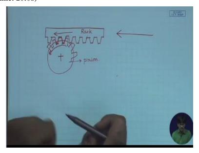
I have rotational motion here and I have put a gear here. This is rotating about this axis of rotation and I have teeth on this. So, I already put a gear on top of this rotating shaft and someone asks me to have linear motion like this. How can I do that? So, for that, one particular example is that I can have something called a rack, a straight sided gear. You have heard of the term rack and pinion, so, we are basically discussing that particular machine element pair.
