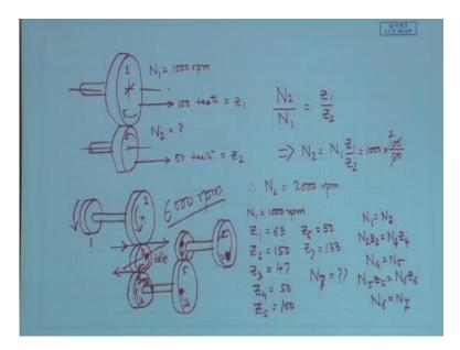
For example, say I have the problem that we were dealing with. This gear is rotating, this shaft is rotating at say let us call it one,  $N_1 = 1000$  RPM and here, we have another gear which is rotating at, this is  $N_2$ , I do not know what is  $N_2$ . But I have been told that this has; just a moment, this has 100 teeth. This is 100 teeth and say this one has 50 teeth. So, what is given?  $N_1$  is given;  $z_1$  is given. So, this is  $z_1$ .  $N_2$  is not given and  $z_2$  is given.
