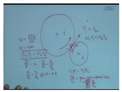
So, if you look at this particular figure, where we are basically representing the gears by circles. So, this is a sort of simplification of the figures. We are saying that if this gear is moving this way, it will make the other gear move this way if it is free to rotate about its rotational axis and therefore, we say that since at this point, gear number 1 is in contact with gear number 2, these 2 are the teeth which are in contact.
