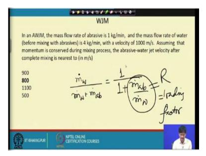
This can be referred to as  $\dot{m}_w/\dot{m}_w + \dot{m}_{abr}$  equal to if you divide this by  $\dot{m}_w$  it becomes  $1/1+(\dot{m}_{abr}/\dot{m}_w)$  and this one is called loading factor or R, loading factor. It is one of the most important parameters in abrasive water jet machining. I intend to include some solved problems and upload it for your use where you will come across the use of such parameters in abrasive water jet machining.
