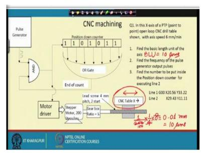
So, let us start right away with our figure that we have come across and the question reads in this X-axis of a point-to-point open-loop CNC drill table shown with axis speed of 6 millimeters per minute, find the basic length unit of the axis? Find the frequency of the pulse generator output pulses? And find the number to be put inside the position down counter for executing line number 2 of this particular couple of lines?
