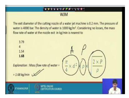
This is A, this is  $\rho$  and this is V, how is V found out? V is found out by converting the pressure energy completely to velocity energy. If you remember we have Bernoulli's equation where P by gamma = V square by 2G = z, so the same thing has been done here, I leave this calculation to you, I am sure you can solve it and this way the mass flow rate can be calculated to be 1.68 kg per minute.
