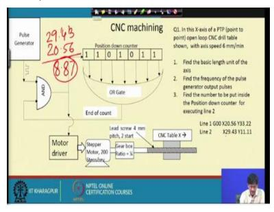
Line number 2 says that I want a movement of 29.43 millimeters, so let us subtract it 29.43 and it was already a 20.56 so this means 13 7 1 14 and this is 6, so this is 8 and 1 goes here 8, 8.87mm of movement are required. So, I have to put some number, so that this will get decremented and it will exactly become 0 when the required motion has taken place. Per pulse I am having  $10\mu m$  of movement.
