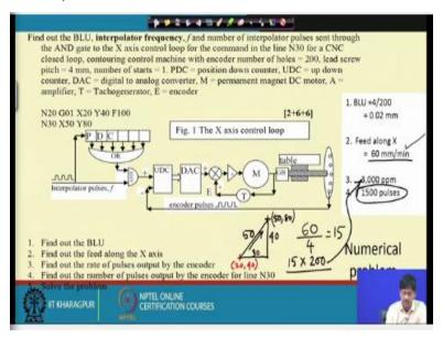
Now this red is which is difficult to this, you are at point 20, 40 and from there you are going to another point 50, 80 50, 80. So, we can easily compute these distances, 20 to 50, 30, 40 to 80, 40, so this must be 40 and therefore this must be 50. So, that means the feed of 100mm is along this path, 100. So, if 50 is here by Pythagoras theorem we can say this is 30, this is 40. So, if 100 is here since feed triangle and displacement triangle they are similar for linear movements.
