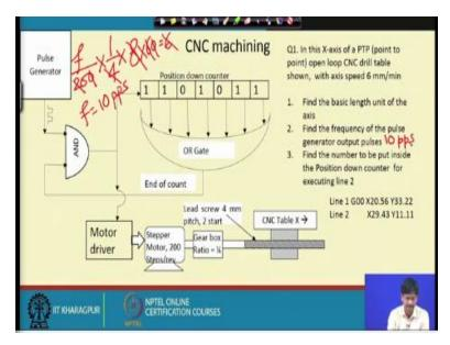
How many of these pulses will give us one rotation? 200 pulses, so these many rotations of the stepper motor will be obtained per second. Now these rotations will be reduced by the gearbox by a factor of one fourth and the amount of motion obtained will be multiplied by the lead of the lead screw and therefore this should be equal to when multiplied by 60 this should be equal to 6 millimeters.
