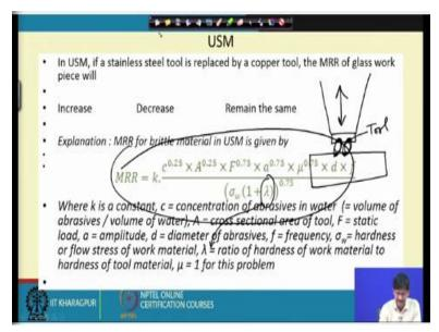
Next, ultrasonic machining. In ultrasonic machining if a stainless steel tool is replaced by a copper tool the MRR of glass workpiece will increase, decrease, remain the same. So, a tool is replaced, remember the tool which was vibrating against the workpiece. Now if steel tool is replaced by copper tool the tool is softer, I have worked it out through this formula but I will give you a physical idea also.
