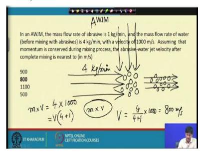
Next, so water jet machining? In case of abrasive water jet machining what are we working with? So, this will be abrasive water jet machining. In abrasive water jet machining the mass flow rate of abrasive is 1 kg per minute and the mass flow rate of water before mixing with abrasives is 4 kg per minute with a velocity of 100 meters per second. Assuming that momentum
