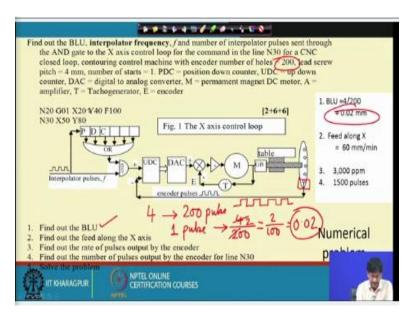
Next UDC up-down counter here, just as we have discussed this thing, so let us go into the problem directly. Find out the basic length unit, how is the basic length unit decided? This is a closed loop system in which we are keeping track of the movement which is taking place. And the encoder sends back pulses; each pulse is therefore our smallest unit of the actual movement carried out. What is this smallest unit?
