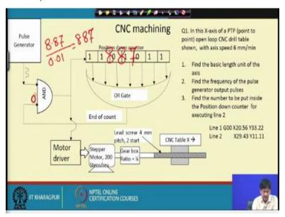
So, this means that if I want to have 8.87mm of movement, how many pulses would be required? 887 pulses will be required in order to get the stepper motor move the table through 8.87mm. So, if we put 887 in binary inside this position down counter, our job will be done. Because while 887 pulses are coming here, 887 pulses will be going there and it will be down counting the contents to 0 and OR gate will put out a 0 here and further pulses will be stopped. So, the number to be put inside is 887.
