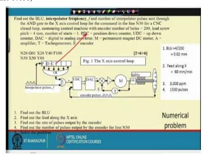
Find out the basic length unit, interpolator frequency f and the number of interpolator pulses sent through the AND gate to the X-axis control loop for the command line 30. For a CNC closed loop contouring control or continuous control, whatever with encoder number of holes 200 lead screw pitch 4 millimeters, number of starts = 1. And PDC stands for position down counter, so this is the thing position down counter.
