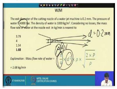
Next, the exit diameter of the cutting nozzle of a water jet machine is 0.2 millimeters, the pressure of water is 4000 bars, the density of water is 1000 kg per meter cube, considering no losses the mass flow rate of water at the nozzle exit in kg per minute is nearest to. These are the options and I am providing the answer 1.68 kg/min. So, let us first see what is the problem about?
