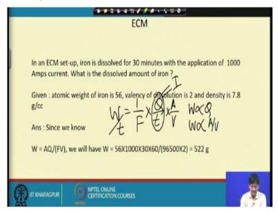
ECM, in an ECM setup iron is dissolved for 30 minutes with the application of 100A current, what is the dissolved amount of iron? So, in this case what we have given is atomic weight of iron is given to be 56, that means gram atomic weight is 56g, valency of dissolution is 2, I have 2
