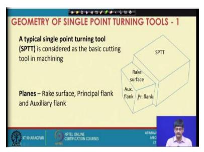
So, first of all on the screen you can see the shape of a single point turning tool, SPTT. So, this is considered to be as the basic cutting tool or cutting element in machining. All cutting tools can ultimately be related to this particular single point turning tool. That is all cutting tools can be ultimately shown to be composed of different single point turning tools or a modification of the single point turning tool.
