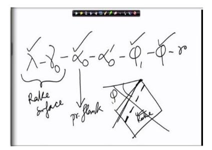
We can define it this way, lambda,  $\gamma_0$ ,  $\alpha_0$ ,  $\alpha_0'$ ,  $\varphi_1$ ,  $\varphi$ , r. You might say is in the same problem that you mentioned about ASA system going to occur here as well, no. Because here you will find that we are defining the rake surface orientation by these two angles. We are defining the principal flank by this one, you might say can the principal flank be defined completely this way; just a single angle is there.
