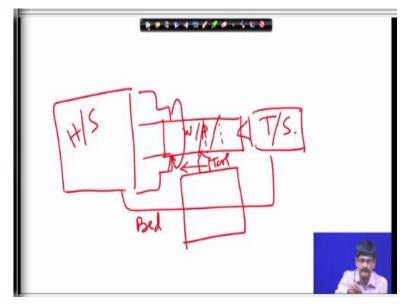
I will just repeat those workpiece, work holding device, headstock, tailstock, basic body of the machine, the lathe bed. On that there is a sort of saddle which can move this way, that way and the tool is typically held on this saddle, I mean carriage. So, this is the lathe bed, this is the tool. So, just see I am going to make the workpiece rotate and the tool is going to move this way, and therefore it primarily describes the helix, the tool describes a helix like that.
