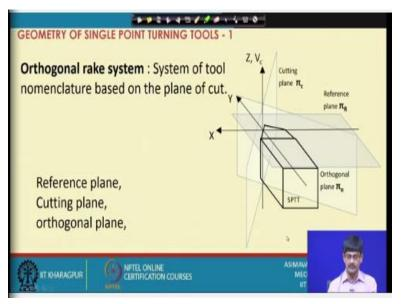
Another one is where the cutting edge, the cutting edge forms the basis of the definition of the geometries that means the angles and the edges etcetera. So, whenever we have cutting edge or other cutting plane based system we call it the orthogonal rake system, what is it? It basically defines a coordinate system where the planes are defined with relation to the cutting edge, in what way?
