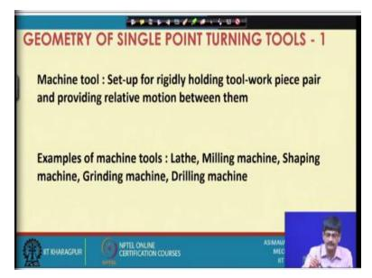
So, the machine tool holds the tool workpiece pair rigidly and provides relative motion between them. The tool that we saw just now is held on the machine tool. Examples of machine tools are lathe, milling machine, shaping machine, grinding machine, drilling machine. Let us have a quick look at some of these machines.
