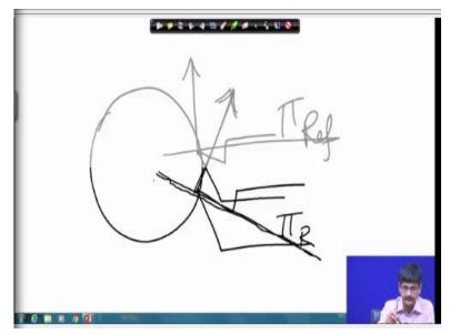
Suppose we are having this as the work piece and this as the tool, in that case the velocity vector will be directed this way. Now suppose someone puts the tool by mistake at a lower height. Suppose this is the tool you have a problem; in that case the velocity vector is this way. And all the tool angles will be changing because the reference plane is now here; previously the reference plane was here.
