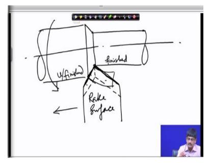
We are looking at the tool from the top, therefore this is the rake surface, where is our job? The job is on this side. It is rotating, the tool is moving this way, so the chips are going to come out as we saw the last day the chips are going to come out here. Over which the chips flow the rake surface and this is the finished part, this is the unfinished part. So, the principal flank is to on this side, we cannot see it from the top but it is there.
