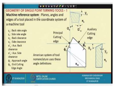
So, let us see the angles which are created by the intersection of these planes with the tool. First of all, I am seeing the tool here from the top, this is the tool from the top. And all angles and planes and edges etcetera are defined in this system of machine reference, it is called the machine reference system. And the American system of tool nomenclature uses these angle definitions, in what way?
