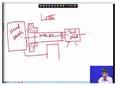
So, for that let us select the white board. On the lathe what kind of machines do we have rather yes? So, on the lathe we have the basic work piece, it is held securely on a device called a chuck or center. So, it is holding onto the workpiece, this one is made to rotate; it has ultimately connection with something called a headstock.
