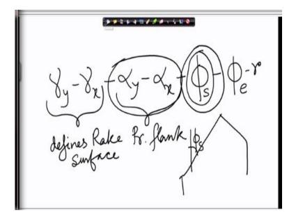
For that in the ASA system in many literature it is given that the tool can be completely defined by this particular nomenclature  $\gamma_y$ ,  $\gamma_x$ ,  $\alpha_y$ ,  $\alpha_x$ ,  $\varphi_e$ , I think it is  $\varphi_s$ ,  $\varphi_e$ , r, we will check this out, r is the nose radius. Now I would not like to follow this particular nomenclature. Because as you would see there are certain problems with this, for example there is no information about the auxiliary flank.
