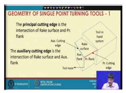
So, after that we come to the definition of the different edges which are present and the different points. Once we have 2 planes intersecting, their intersecting edge can easily be identified and here we have identified the intersection between rake surface and principal flank as this line, this red line and we have named it as the principal cutting edge. In the same way the rake surface and the auxiliary flank will also have an intersection that is called auxiliary cutting edge.
