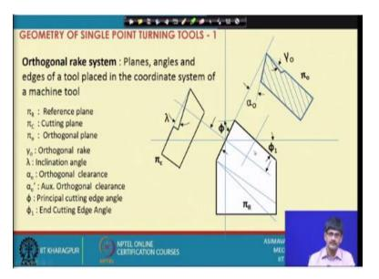
And let us see how the sections come out to be in that case. The sections I mean the angles, first of all if you look at this figure this is the cutting edge, once again this is the cutting edge. Where is the cutting plane? The cutting plane is appearing as a line here, it cannot be seen from the top. As it is a vertical plane it cannot be seen from the top but here it is appearing as this is the trace of the cutting plane.
