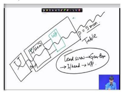
I will draw the simplest possible description, this was the lead screw, it was at an angle. So, if we had the lead screw it must have been traveling on a nut which had a pitch, so let us say this pitch is equal to say P or say 5 millimeters. So, if the lead screw has a pitch of 5 millimeters per rotation it will make the table travel, so this is the table, the table will be traveling per rotation by distance of 5 millimeters.
