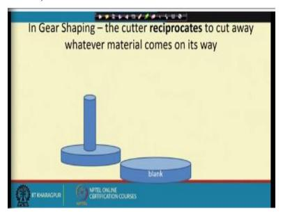
So, now we come to the idea of gear shaping. Gear shaping can be explained in just one sentence, while 2 gears are rotating, if these 2 are rotating together if one is a solid and the other is made to reciprocate, this one will remove all the material it meets on it is way and what will result is the actual gear. So, there is a solid material and this one is a perfectly made gear, they are made to rotate together that is you are giving them individually rotations.
