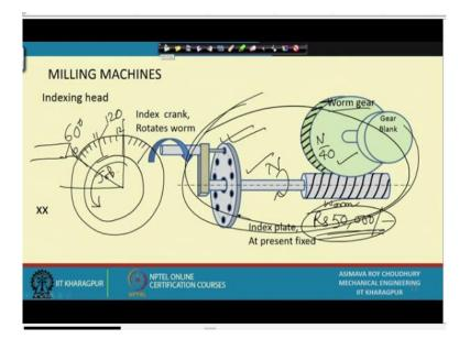
Milling machines, first of all the indexing head, what is this indexing head that we are talking about. First of all, let us see; what is our ultimate end use? This is a gear blank, it might be something different, it might be a cylinder on which we want to cut 4 sides at equal intervals, it might be say a hexagon to be produced from a cylinder or it might be as we have indicated a gear blank.
