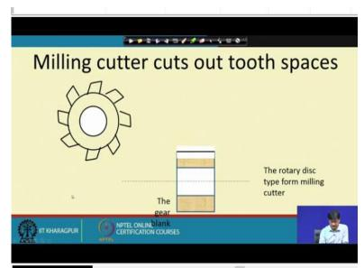
Next we will come to this one I would like to show you something first. How does a gear cutter cut out those spaces? So, this is the cutter and this one is the gear blank where the cuts will have to take place this way. Here what we intend to do is in the other view this, if you look at it this way, you will be seeing a smooth circular body and we have to cut the teeth this way and this is going to cut it right through and go back.
