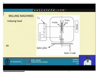
The possible solution is this, first of all see what we were talking about, this is the index crank, this index crank was being rotated, we are seen in a different perspective, we are seeing it from the top. This index crank rotates, this rotates the worm, this rotates the worm gear and this is your gear blank. Now what we do is we extend this shaft connecting the worm gear with the blank backwards and take a feedback we pass it through a gearbox remember gearboxes.
