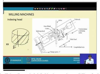
This gives us I will just discuss in brief, this gives us the possibility of using the indexing head and the universality of the milling machine; that means, the ability to rotate about a vertical axis to carry out a machining process called helical milling. What is helical milling? Helical milling means the ability of the milling machine or the application of the milling machine to cut a helix.
