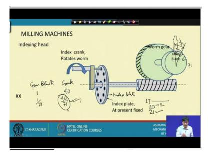
Four times, I want to rotate by 90°. So, once again we say 90° of movement; that means, how much, blank and crank. Crank means this handle which is moving round and round here. So, if I have to move by one fourth of a rotation I must be moving 40 by fourth of a rotation. Remember 1 rotation, 40 rotations, one fourth rotation 40 by 4 rotations unitary method.
