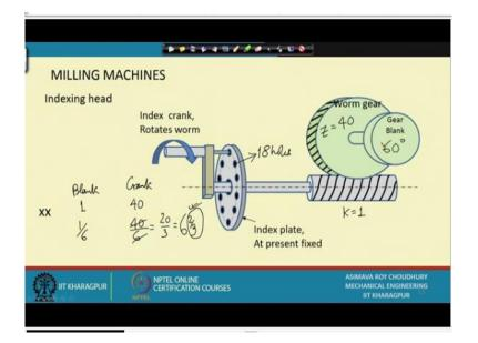
In what way I choose a worm with say k = 1, number of starts equal to 1 and this one with number of teeth equal to 40. Therefore, have if the blank rotates once this crank has to rotate 40 times in order to implement it. I rotate here 40 times, the worm rotates 40 times, this will only rotate once. So, I magnified the amount of rotation which is there on the blank; blank 1, crank 40 times.
