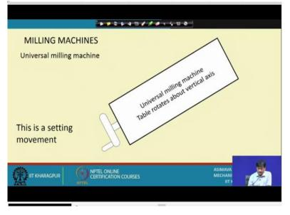
Let us see how the universal milling machine is working; how it operates? And mind you this is a setting movement. During machining generally, the universal milling machine table does not rotate about the vertical axis. So, this is the rotation that we are talking about; looking from the top you can set it to any angle that you want.
