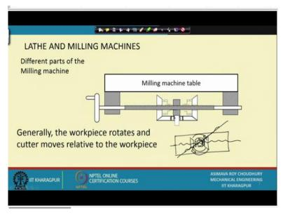
Looking from the top we have this to be the table; this to be the screw, these to be the bevel gears and they are rotating on top of another bevel gear and inside there is the nut and on this side there is the clutch. So, even if this thing changes; this moves this way, this moves that way, the screw comes here; everything still remains in contact, so this way we are taking care of it.
