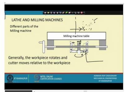
This is a possible configuration of what is going on inside; first of all, let us locate that nut that we were talking about; this is the nut and what is the nut doing? The screw is passing through it and therefore, the nut being held steady somewhere; it is making the table move. So, the table will be suffering motion like this; what are these things on the sides? These are bevel gears.
