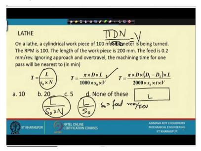
Next on the lathe a cylindrical work piece of 100 millimetre diameter is being turned; the RPM is 100, the length of the work piece is 200 millimetres, the feed is 0.2 millimetres per revolution, ignoring approach and over travel the machining time for one pass will be nearest to in minutes 10 minutes, 20 minutes, 5 minutes, none of these. So, here first of all what is approach and over travel?
