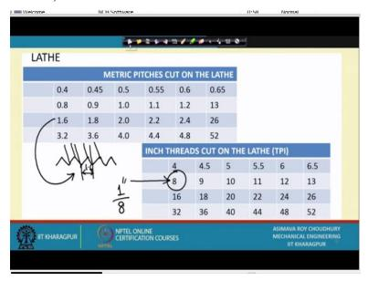
And in fact you will notice that there might also be 2 such charts in which metric pitches are given which means sorry. These are the threads which can be cut and they mean to say that if this is a thread etcetera. In that case this if you want this to be say 1.6 they will say that set up the gears in a particular manner which I have not shown up till now and you will get 1.6 pitch.
