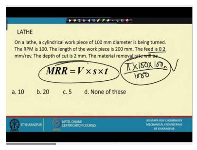
So, on a lathe a cylindrical work piece of 100 millimetres diameter is being turned. The RPM is 100, the length of the work piece is 200 millimetres. The feed is 0.2 millimetres per revolution.
