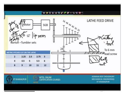
So, on the lathe we have already come across the basic motor which is providing power or to all the processes in the machine except if you are giving manual feed, but otherwise it is providing all the power and we had that speed gearbox which is leading on to the spindle which has not been shown for simplicity. So, this leads to the spindle I will write it down, so that you will remember this will do spindle.
