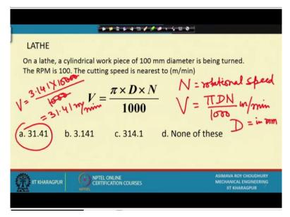
To start with on the lathe a cylindrical work piece of 100 millimetre diameter is being turned the RPM is 100, the cutting speed is nearest to in meters per minute, 331.41, 3.141, 314.1 and none of these. So, in many cases what happens is when a student is first getting to know about cutting speed there is confusion about what is cutting speed and what is rotational speed. Rotational speeds say we refer to as N, N = rotational speed.
