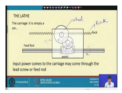
This is the way in which the apron mechanism of the carriage operates. So, what is the carriage? It is a car; it is simply a car nothing else, then where is the wheel of the car? This is the wheel of the car, this one; wheel. Where is the road? This is the road; this rack is the track of the wheel. So, how does it move? You know this is the feed rod by the same mechanism as we have discussed it has a keyway inside it and on that fits a worm I will explain what a worm is.
