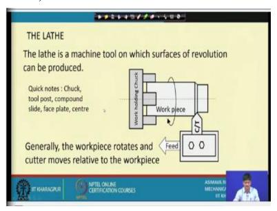
So, first of all the lathe is a machine tool on which surfaces of revolution can be produced. That is, I can make a cylinder, I can make a cone, I can make a flat surface by which is also a surface of revolution, I can make grooves, I can make threads, I can make frustums of cones. I can make curved surfaces also, so all these which are surfaces of revolution they can be produced on the lathe.
