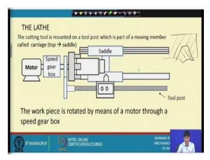
In the next slide what we see is, now the upper part of the carriage called the saddle just like we put a saddle or seat on the back of a horse on top of the lathe bed seen from the top. The basic body of the lathe we have put a saddle like element. So, this one is containing the tool then why not what is the lead screw doing? Lead screw is simply passing through the carriage and we may or may not connect to the lead screw to derive power.
