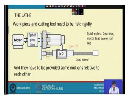
This is you know we are going on adding, so with this add on process ultimately we will be getting the full picture of the lathe. Here comes the prime mover, the motor, from the motor in order to rotate the workpiece; we see that we have put something in between, what is this? This is called a speed gearbox, what is its utility? You know we might not always want to rotate the workpiece at a particular rpm; we might be changing this rotational rate.
