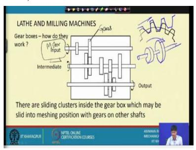
This is a more detailed figure of the gearbox that we were naming just now. What is the gearbox? You know just like we have speed gearbox and feed gear box; they have some machine elements inside. So, that if they are shifted from one position to the other; we would be attaining different output rotations of the gearbox. So, which is the input and which is the output?
