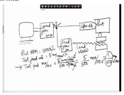
So, let us first of all select fresh page in which we start with, here we had the motor, from the motor there was the shaft and we had the gearbox, speed gearbox. From the speed gearbox we had a bifurcation, power was going this way and it was serving the tool, so this is called feed
