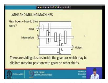
So, this is the way in which it can be slid or it can come back also, you can have this position as well as that position. Now why have we shown 3 shafts? Because by shifting it from here to here I can get different speed ratios, these 2 gears will have different teeth ratio, and these 2 gears will have different teeth ratio and they will give rise to different speeds on the intermediate shaft.
