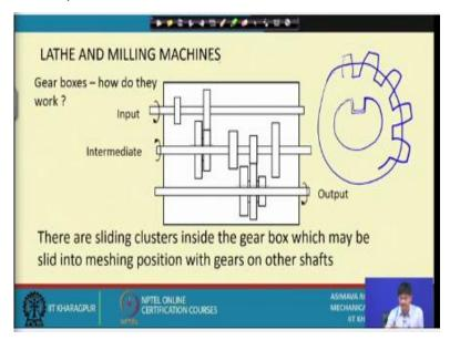
So, this is the input shaft, it is rotating due to its connection with the motor, and these are 2 gears on it. This one is another gear I mean a set of gear 2, a pair of gears which is sometimes referred to as sliding clusters, so this is a sliding cluster. What does it do? It can slide along the shaft but still maintain rotational connection. That means if the shaft rotates, the sliding cluster has to rotate the other way if the sliding cluster is rotating it will make the shaft rotate.
