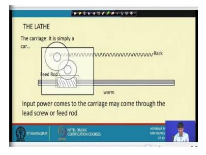
That is it, it simply moves this way, so this is how the carriage is working. So, this mind you is the feed rod not the lead screw, the lead screw is just by the side of it in order to maintain simplicity I have removed it. I have also removed the mechanisms for automatic feed mechanism for foolproof arrangement, mechanism for cross feed all these things I have removed for maintenance of simplicity.
