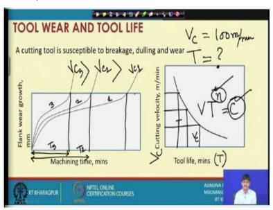
Next, so if we develop such flank wear curves, in that case if we use different values of cutting velocity. Suppose I am using cutting velocity 1, I reach the 0.3 mm at this particular time. If I use cutting velocity 2, I reach this particular limiting flank wear say 0.3 m at this particular time. So, this way if I use cutting velocity 3, I reach that particular limit here. What is the relation between these cutting velocities?
