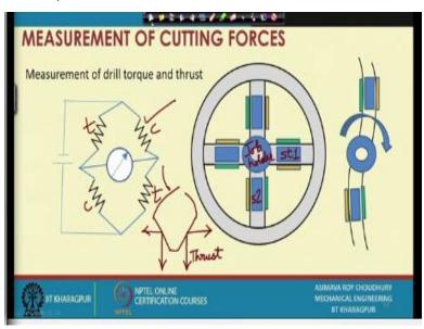
In a similar fashion, we can also have drilling dynamometers. In the drill if you have perfectly made cutting lips of the drill which are symmetric about the central axis, there would be no forces will be balanced in the radial direction, what do I mean by this? Suppose this cutting lip is experiencing this force and it is experiencing that force. So, in that case this will also be experiencing this force, and an opposite and hopefully equal force in this direction.
