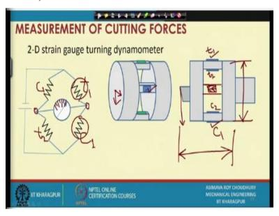
So, to start with, when we were talking of measurement of cutting forces, we discussed the theory of strain gauges and this fact that the strain gauges have a compact. So, we had discussed the theory of strain gauges and understood that dr/r divided by the strain = gauge factor was roughly equal to 2, which showed that there is a relation of proportionality existing between resistance change and strain.
