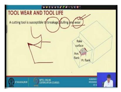
Today's actual discussion was on tool wear and tool life, what do we mean by this? Tool wear means that whenever a tool is being used for removing material, after a few minutes of use if you take out the tool and look at the tip of the tool which is defined by the intersections of the principle flank, auxiliary flank and rake surface. We will notice that it has undergone a change, why so? This is because the tool will be a deteriorating in quality when it is being put to use.
