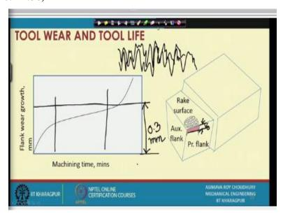
Generally, we are more interested about this flank wear growth. Flank wear growth has a limit after which we generally do not use these turning tools. I mean for that matter all tools, say in case of we keeping our discussion restricted for the time being to turning tools now. So, what happens is when the average flank wear, what do we mean by the average wear? It is not that notch, it is something to do with, this value perhaps average flank wear and we sometimes call it  $V_b$ .
