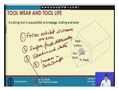
Forces exhibit increase over time, then other things might also happen, suddenly you find the surface finish which is obtained on the workpiece, it is not acceptable, it is deteriorating. There might be vibration and chatter, there can be increase in power consumption etcetera, there can be increase in the sound, there can be too much heat coming out from the colour of the chips etcetera, it can be found out.
