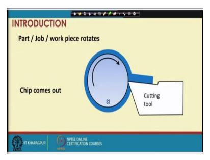
So, let us have a look at how this whole thing can be done on the lathe, the lathe is the most common machine tool. On that surfaces of revolutions are produced, surfaces of revolution mean that about an axis the body will have a symmetric shape, axis symmetric bodies are produced, what is this body? For example, just one moment, this body is a cylindrical body seen from the end, so this is the axis of rotation, it is rotating this way.
