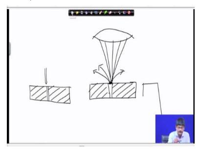
Non-conventional machining, say I will start with laser I need to make a very narrow hole here, what kind of dimensions am I talking about? I am talking about say dimension of say 250 microns; if it is 250 microns it means it is 0.25 millimeters. Now is it possible to drill a hole of 0.25 millimeters by conventional means, that means by mechanical means, having a tool which can push away material and cut it off and produce this hole, maybe it is possible.
