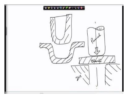
This is a very simple and explanatory example, someone shows you this part which is a sheet metal and we are seeing it only from the side sort of sectional view but how was this done? And that particular person says that it was done by say deep drawing, what is deep drawing? So, initially there must have been a body of this type, a sheet metal piece may be circular, circular this way and there was a punch and there was die.
