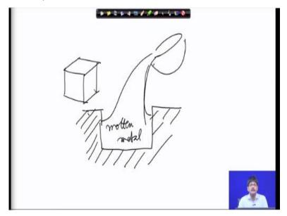
Suppose I have a cavity, I am showing very simple principles, so some material is here, so that a cavity is formed. Inside this cavity I pour molten metal, so ultimately the molten metal will solidify. So, if it solidifies it will attain the inside or internal shape and be of a definite size, so this is casting. Melt the material; pour it into a cavity of predetermined shape and size.
