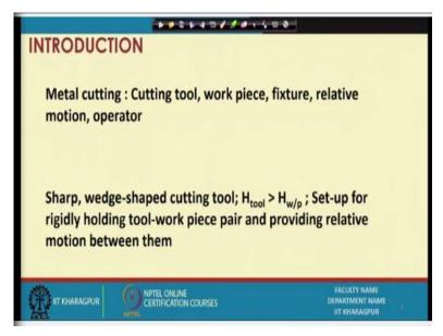
So, if you have a look here, metal cutting involves cutting tool, workpiece, fixture, relative motion and in many cases operator, what will be exactly mean by this? We mean that just like we were having some active member which was removing material from the workpiece or the blank. In case of metal cutting we have something called the cutting element or cutting tool which actually removes material by dint of its higher hardness by a presence of a sharp edge, at least 1 or 2 sharp edges on it.
