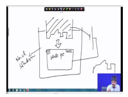
You have the part here and you are having a job of this type. And you bring it towards the job; you give it electrical connection; you submerge the whole thing in electrolyte solution say NaCl solution. This is your workpiece at this moment, it is the blank. So, the conjugate of this surface will be produced because other parts like this protruding part it will be dissolving electrolytically, this will be dissolving, this will be dissolving etc.
