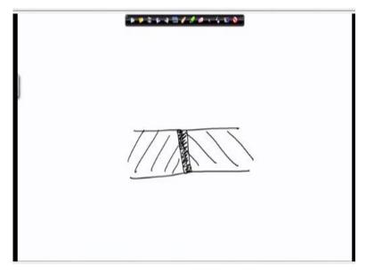
So, if I have two such materials, this is one, this is the other and I heat them at this point, so that this part melts, that is it. This part melts when it solidifies this will be a single piece, so that we can join parts and make up shapes. Our main concern is to make shapes of predetermined shape and size. So, many times you might have seen even in civil activities, gates, grills, window grills etc., these are made very elegantly by welding.
