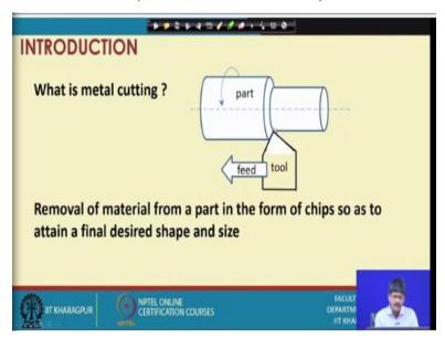
If you look at this particular figure what do we have? We have here a work piece or part or job shown here rotating. And there is something called a tool or a cutting tool here and how is it characterized? It is characterized by a sharp point and some sharp edges here and it is moving past the rotating member that is removing material.
