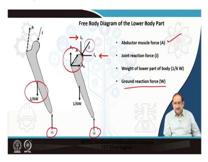
Now, let us go to the free body diagram of the lower part of the body. In this free body diagram, the forces that are taking part are the abductor muscle force which is given by here; the joint reaction force J, which can have two components along X and Y direction; the weight of the lower part of the body which is 1/6th of W and the ground reaction force which is given by W. The ground reaction force actually is the reactive force which is equal to the weight of the body.
