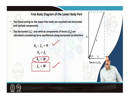
Considering the free body diagram of the lower part of the body, the forces acting on the lower free body diagram can be resolved along the horizontal and vertical directions. And thereafter, we can consider the force equilibrium along the X direction, and we can easily write down the mathematical relationship between the abductor muscle force along X direction and the joint reaction force along X direction. So, we get basically Jx equal to W, because Ax has been earlier calculated as W.
