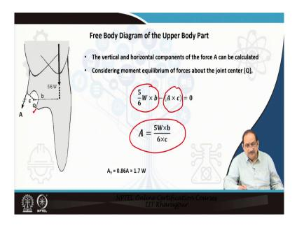
Now, considering the free body diagram of the upper part the body, the vertical and horizontal components of the force A can be calculated. Then considering the moment equilibrium of forces about the joint center Q, we can actually write the two moments: one due to the gravitational force, the other due to the abductor muscle force. So, A, abductor muscle force can be calculated in terms of body weight and the dimensions of the lever arm b and c.
