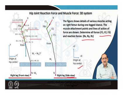
Let us now consider a 3D system. Now, we will consider the hip joint reaction force and muscle forces considering a 3D system. Earlier we have used a two dimensional system. Now, it is a 3D system, and we will be using the vector mechanics method to find out the forces muscle forces F1, F2, F3, and the joint reaction forces Rx, Ry, Rz.
