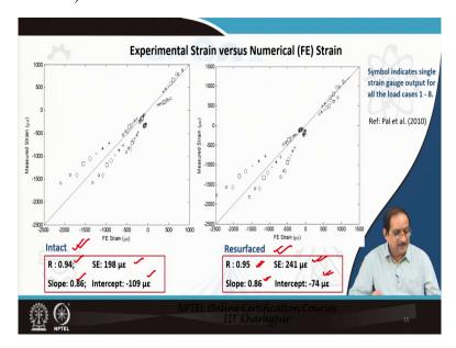
Let us come to the results. The results are actually presented in the form of comparison between experimental strain and numerical or FE predicted strain. So, on the left, we have the results corresponding to the intact femur, and on the right, we have the results corresponding to the resurfaced femur. In the figure, one symbol indicates single strain gauge output for all the load cases from 1 to 8. There are eight load cases. So, each symbol corresponds to a single strain gauge output.
