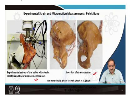
Now, let us discuss about the experimental strain and micromotion measurements on a pelvic bone. On the left, you can see the experimental setup of the pelvis with strain rosettes and linear displacement sensors. So, the linear displacement sensors are oriented along mutually orthogonal directions. So, LDS 1, 2, and 3 are oriented along three perpendicular directions. On the right, we have the location of strain rosettes fixed on the surface of the composite pelvis or composite pelvic bone.
