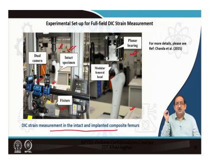
The experimental setup for the full field DIC measurement is presented here. On the left, we have the intact specimen, we have the dual cameras, and of course, the fixture on which the bone is fixed and the loading mechanism that we have used earlier is used here to apply the vertical load.
