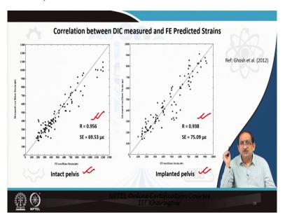
Now, we compare quantitative values of DIC measured strains and FE predicted strains. For the intact pelvis and the implanted pelvis, we can compare the DIC measured and FE predicted strain and you can clearly see the high correlation between the measured strain and the FE predicted strain for both cases.
