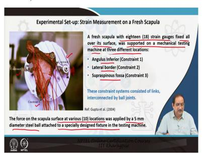
Now, I would like to discuss about strain measurement on a fresh sample of bone and that sample of bone is a scapula. So, it is a fresh sample of bone taken out from donated cadavers and this had been used for experimental validation of a finite element model. Now, fresh scapula with 18 strain gauges is fixed all over its surface.
