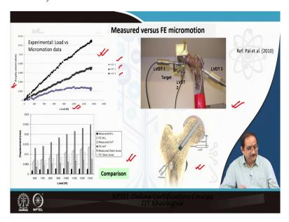
Let us now present the results of measured micromotion versus the FE predicted micromotion. On the left, you can see the experimental data. So, we have the load on the x-axis and the micromotion or displacement recorded by the three LVDTs 1, 2, and 3 presented here in the graph.
