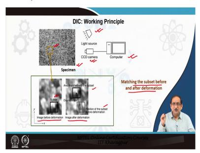
Let us briefly discuss about the working principle of the digital image correlation technique. So, as indicated earlier, you can see that there is a white light source, the digital cameras to record the deformation of the speckle pattern and the digital cameras are connected to the console or the computer.
