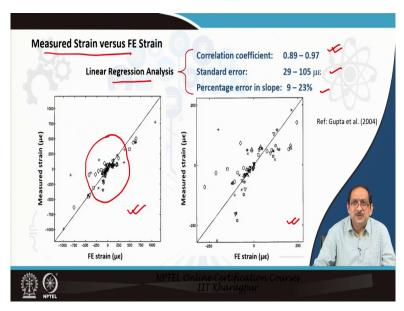
Now, let us compare measured strain and finite element strain as indicated in the figure. So, the figure on the left, as you can see here, consists of all the measured data, but the figure on the right is plotting a zoomed view or closer view of a cluster of data in the range of  $\pm$  250 micro strain. So, that is in the low range of  $\pm$  250 micro strain.
