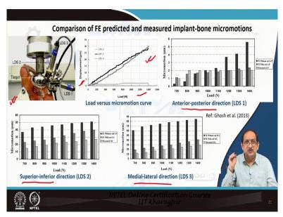
Let us now compare the FE predicted and measured implant-bone micromotion. So, we have measured the micromotions or displacements against load, and the load versus the micromotion curve is presented here in the slide, based on the experiment performed here.
