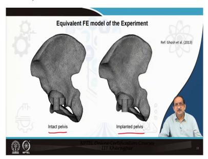
The equivalent FE model of the experiment was developed, as you can see here and now presented in this slide for the intact pelvis and the implanted pelvis.
