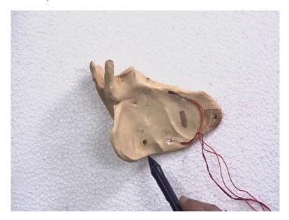
Let me present to you a plastic model of a scapula, a plastic model of scapular on which you can see two strain gauges fixed on the surface of the scapula. This plastic model was used as a pilot study before the measurements on a fresh sample of scapula were undertaken. Here you can see two holes, one on the angulus inferior and the other in the fossa area, through which the supporting link mechanisms are attached.
