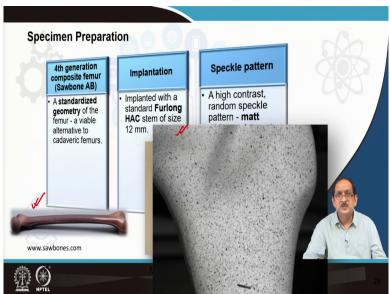
Next, we will be discussing about testing the femur with a total joint replacement femoral component. Now, quickly we will go through the specimen preparations; as you can see, we use the fourth-generation composite femur from sawbones. We actually do the implantation by taking help from an orthopaedic surgeon and following the standard surgical procedure.
