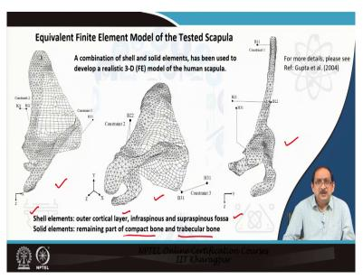
So, after the experiment was carried out, we actually developed an equivalent finite element model of the tested scapula. So, in this slide, you can see in three views the finite element model of the tested scapula. A novel approach, a combination of shell and solid elements, was used in the study, which was particularly appropriate to develop a realistic 3D finite element model of the human scapula.
