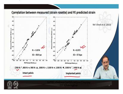
Let us come to the results that is the correlation between the measured strain and the FE predicted strain. So, here we have several load cases as indicated from 700 to 1400 in steps of 100 Newtons. We have increased the load and we have recorded the measurement as well as we have calculated the FE strains at comparable locations.
