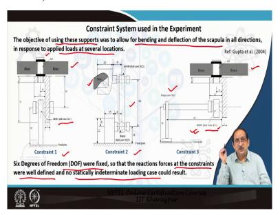
Let us discuss briefly about the constraint system used in the experiment. The objective of using these supports or constraint systems was to allow bending and deflection of the scapula
