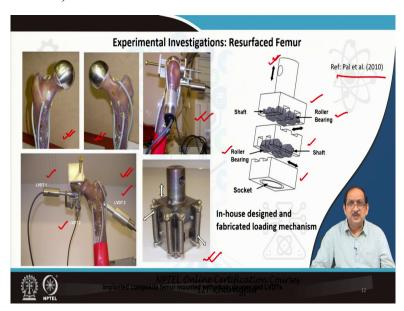
In this slide, we will be focusing on the resurfaced femur. So, as you can see in the figure, on the left, the two figures facing opposite to each other are photos from the experiment, and here you can see the strain gauges are fixed at different locations on the implanted femur. Now, apart from the strain gauges, there were LVDTs, linear displacement sensors to measure displacements or relative displacement between bone and implant.
