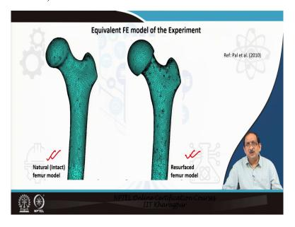
Now, after performing the experiment, we have developed the finite element models of the intact femur and the resurfaced femur. This is actually an equivalent finite element model of the experiment.
