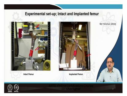
So, let us now see the experimental setup where we tested. You can see the loading fixture and the intact femur is fixed or positioned, maintaining the anatomical angles and it is held in a mechanical testing machine. On the right, we have the implanted femur and this is also held in a similar way with the load application mechanism on the top.
