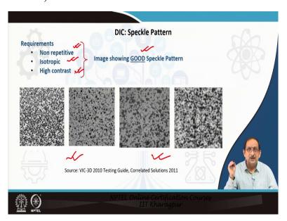
Now, in this slide, images of some good speckle pattern are presented. As you can see, the requirements are a non-repetitive type of randomized speckle pattern. The speckle pattern should be isotropic and have high contrast, as indicated in the four images. So, this sort of good speckle pattern is expected to give desired results using the DIC technique.
