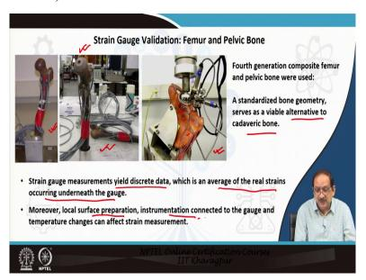
Now, we will be discussing about strain gauge validation on the femur and pelvic bone, both intact and implanted bone structures. Now, with time fourth-generation composite bones have evolved, and they have been commonly used in experimental investigations of biomechanical structures like implant and implant-bone structures.
