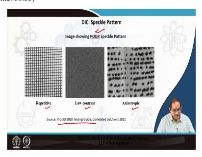
The quality of the generative speckle pattern has an important influence on the results of the DIC technique. Now, in this slide, the image shown here are examples of poor speckle
