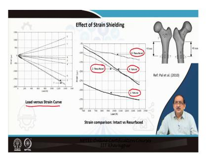
The effect of strain shielding is evident from the experimental measurements, as you can see here in the slide. So, the load versus strain curve is plotted for eight strain gauges, as you can see here. Now, we will focus our attention on strain gauge 2, so it is located exactly at similar positions.
