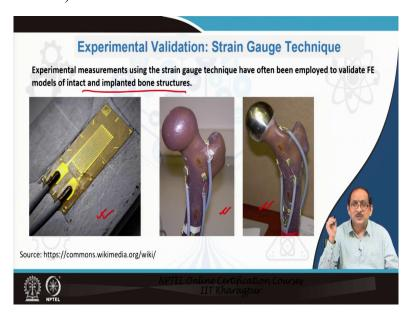
Now, let us move into the second topic, which is on experimental validation using the age-old strain gauge technique. Now, experimental measurements using the strain gauge technique have often been employed to validate FE models of intact and implanted bone structures. So, as you can see, in this slide on the left, we have a typical strain gauge that is generally glued
