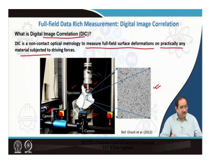
We will now move into the third topic, which is quite interesting. This is regarding the full field data rich measurement using the digital image correlation technique. Now, what is digital image correlation? DIC is a non-contact optical measurement technique to measure full-field surface deformations on practically any material subjected to driving forces or subjected to loadings.
