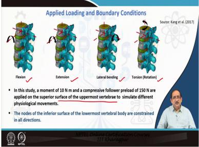
Now, let us come to the applied loading and boundary conditions. The movements of the spine consist of flexion, extension, lateral bending and torsion or rotation. Moment of 2.5 to 10 N-m along different directions and a compressive follower preload of 150 to 1200 N is generally applied on the superior surface of the uppermost vertebra to simulate different physiological movements, as observed in earlier studies.
