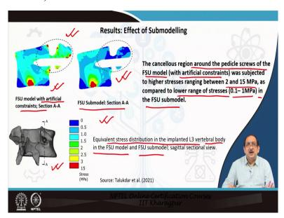
Let us discuss the results on the effect of the sub modelling technique. Now, as you can see here, the evaluation of stresses and strain adjacent to the fixed boundary condition of the small spinal segment appears to be inappropriate and may lead to doubtful results. The artificial constraints generated high stresses, as shown in the encircled region in the figure.
