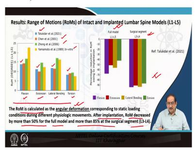
Let us discuss the results predicted by the intact and implanted lumbar spine models, and we will be comparing the predicted results from our study with some earlier published studies. So, the range of motion, calculated as the angular deformation corresponding to static loading conditions during different physiological movements as you can see flexion, extension, lateral bending, and torsion is presented here on the left.
