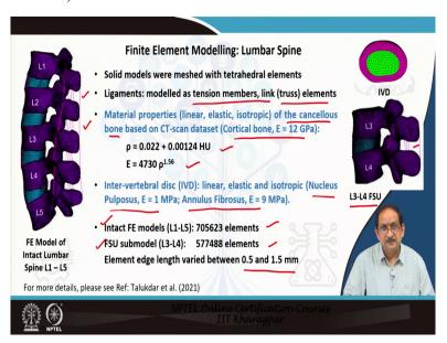
The finite element model of the lumbar spine was created by meshing a solid model with tetrahedral elements. The ligaments were model as tension members; truss elements as shown in the figure presented on the left and also on the line right. Now, the material properties of the cancellous bone were based on the CT scan data set, whereas the cortical bone which was segmented was assigned a material property, Young's modulus equal to 12 GPa.
