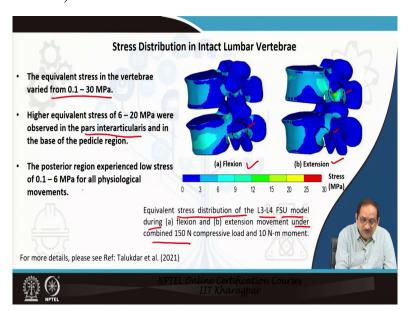
The stress distribution in the intact lumbar vertebra is presented in this slide. The equivalent stress distribution in the L3-L4 FSU submodel during flexion and extension movement under a combined load of 150 N compressive force and a moment of 10 N-m is presented.
