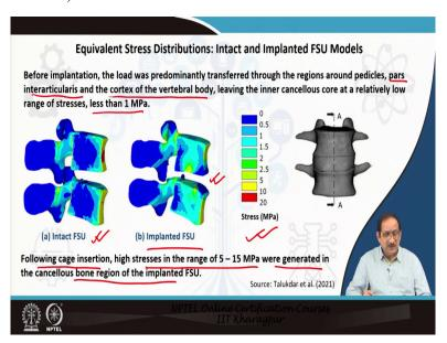
Let us now compare the intact and implanted FSU models. Before implantation, the load was predominantly transferred through the regions around pedicles that is pars interarticularis and the cortex of the vertebral body, leaving the inner cancellous core at a relatively low level of stress, less than 1 MPa, as indicated here in the figure.
