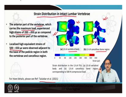
Now, let us look into the detailed stress and strain distribution. First, we are presenting the strain distribution in the intact lumbar vertebra. So, the anterior part of the vertebra, which carries the maximum load, experienced high strains, 200 to 450 microstrain as compared to the posterior part of the vertebra, which experiences less strain.
