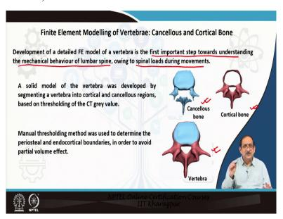
Now, finite element modelling of the vertebra involves some detailed modelling procedures. It has been observed in some earlier studies that the cortical and cancellous bone regions of the posterior part of a vertebra are modelled as a single unit, and a common material property is assigned to the posterior region of the vertebra.
