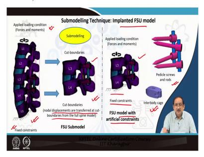
Now, let us again employ the sub modelling technique for the implanted FSU model. As you can see here, we have the implanted model full model with applied loading conditions, forces and moments and fix constraints at the inferior end of L5. We also have FSU submodel of L3- L4, and the nodal displacements are transferred at the cut boundaries from the full lumbar spine model to this sub-model.
