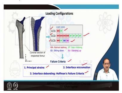
The loading configurations used in this analysis actually vary, there are three loading configurations LC 1, LC 2 and LC 3 and we are now going to investigate the effect of different loading configurations on the failure criteria and the stress-strain distribution. So, loading configuration 1, consists of two load cases. It is the maximum load cases during heel contact of normal walking and stair climbing.
