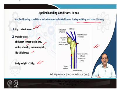
Here we present the applied loading conditions that include musculoskeletal forces during walking and stair climbing only. So, we have used data for our model. So, we have hip contact force and muscle forces like abductor, tensor fasciae lata, vastus lateralis, vastus medialis, illo-tibial tract and these quantitative values of forces will be dependent on the patient body weight.
