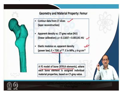
Now, let us present to you a summary of the geometry and material property of an intact femur. So, we start from contour data of CT slices, using layer reconstruction method was called we develop the finite element model, and from finite element model, we apply the linear calibration of apparent density with respect to the CT-grey value.
