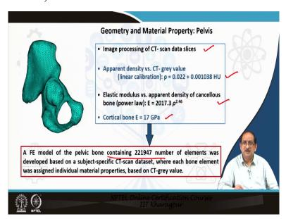
Now, this slide summarizes the geometry and material property, and finally, the development of the FE model of a pelvis. So, it starts from image processing on the CT slice. And then, using the linear relationship between apparent density and CT-grey value and power-law relationship between apparent density and Young's modulus, we can actually obtain a heterogeneous model of bone.
