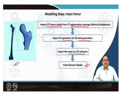
Now, we discuss the modelling steps corresponding to an impact femur for example. Now, we import the STL model of the femur from the segmentation package, and then we export the STL geometry for FE mesh generation. Then, we export this mesh to a finite element software that you may be using.
