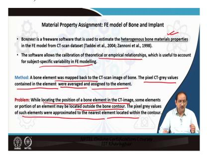
Now, BONEMAT is a freeware software that is used to estimate heterogeneous bone material properties in a finite element model from CT scan data. Now, this is a freeware software that can be used in combination with finite element software, for example, ANSYS, and we have used it successfully in allocating bone material properties. The software allows the calibration of theoretical or empirical relationships, which is helpful in account for subject-specific variability in the FE model.
