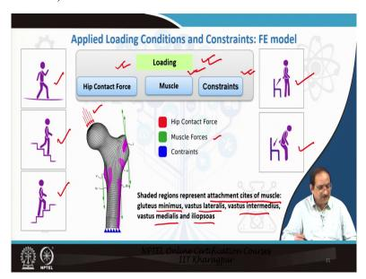
Now, let us come to this lecture's third and final topic on applied boundary conditions and constraints in the FE model. So, we need to load the FE model. So, here we consider the femur, hip contact force, muscle force and constraints as indicated in the slide is presented here.
