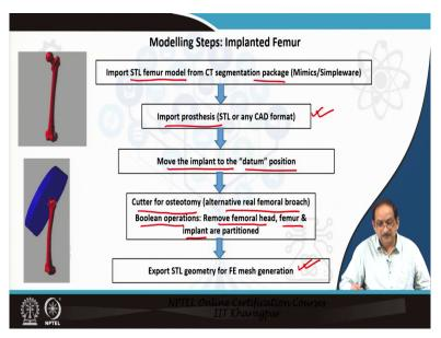
Now, the modelling steps for the implanted femur may be a little bit more complex as compared to the intact femur. So, here also we import the STL femur model from the segmentation on image processing software. We separately import the prosthesis's STL or CAD file and move the prosthesis to the specific position or the datum position as required in the surgical technique.
