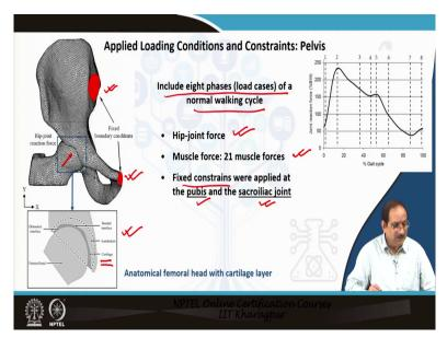
Now, applied loading conditions and constraints for the pelvis, this model was created by us. So, you can see that this applied loading condition included eight phases, load cases of a normal walking cycle. So, we have a set of data corresponding to hip joint force, 21 muscle forces for each load case. And please pay attention here that about the fixed constraints applied at the pubis and the sacroiliac joint in the finite element model.
