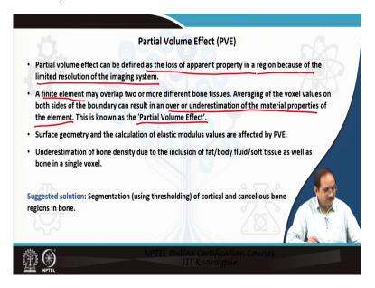
This problem, generally known as the partial volume effect, can be defined as the loss of apparent property in a region because of the limited resolution of the imaging system. A finite element may overlap two or more different bone tissues averaging the voxel values on both sides of the boundary, which can result in an overestimation or underestimation of the material properties of the element.
