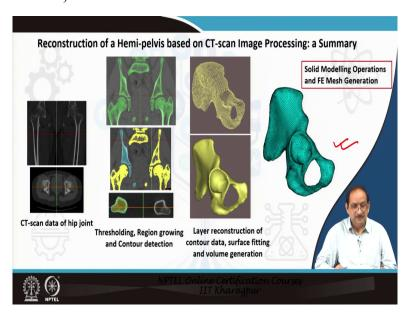
A similar summary can be seen here. So, this is a Hemi-pelvis. So, the earlier slide was on the femur, intact femur. This slide is on the FE model of the Hemi-pelvis that has been generated using an exactly similar procedure.
