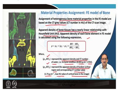
Let us now come to the second topic of this lecture on material property assignment in the FE model of bone and implant-bone structure. The assignment of heterogeneous bone material
