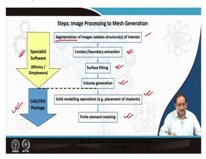
Now, let us talk about the steps from image processing to mesh generation. So, these are the critical steps. The first step is the segmentation of images. So, segmentation of images isolate structures of interest. Then we detect the contours, so contour detection or boundary extraction, then apply a surface fitting and obtain a volume.
