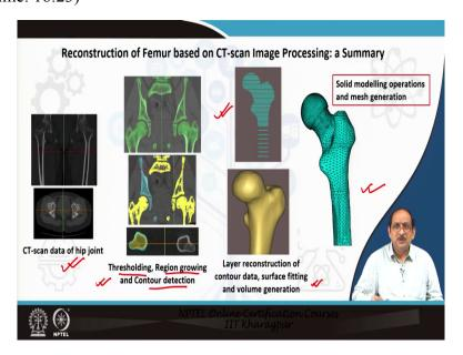
This slide presents a summary of the reconstruction of the femur based on CT scan image processing. As you can see, it started from CT scan data of the hip joint from which we apply the image processing techniques like thresholding, region growing, and contour detection.
