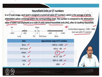
Let us now discuss Hounsfield units or CT numbers. In a CT scan image, each pixel is assigned a numerical value or CT number, the average of all the attenuation values contained within the corresponding voxel. Now, this number is compared to the attenuation value of water and displayed on a scale of units known as the Hounsfield units or HU and it is named after Sir Godfrey Hounsfield.
