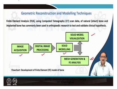
Now, let me start with the geometric reconstruction and the details of the modelling techniques. Finite element analysis using computed tomography scan data, popularly known as CT scan data of natural as we refer to natural intact bone and implanted bone, has been commonly used in orthopaedic research to test and validate the clinical hypothesis. So, finite element analysis has been used in orthopaedic research to test and validate the clinical hypothesis.
