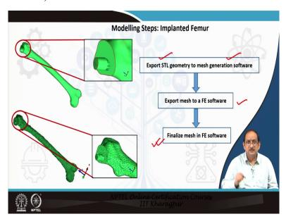
We just discussed it a little bit more in detail. Here you can see exporting the STL geometry for mesh generation. Then, we export the mesh to a finite element software. And here, we evaluate the FE mesh, and if there is some rectification required, we attend to it and finalize the mesh quality in the finite element software and finalize the finite element model of the bone.
