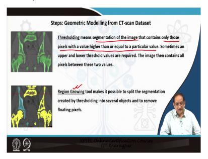
Now, let us discuss a little bit more detail about geometric modelling from CT scan data. So, thresholding is the first operation that we apply on a CT scan data slice. So, thresholding means segmentation of the image containing only those pixels with a value higher than or equal to a particular value. So, it is a threshold value based on which we segment the image.
