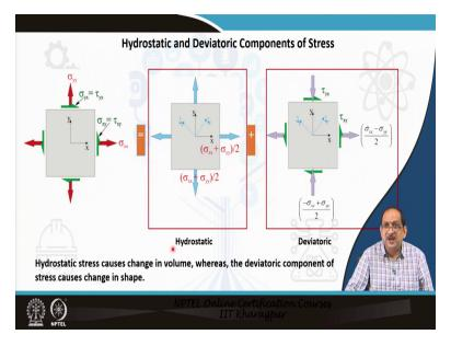
Diagrammatically, the state of stress can be represented as a hydrostatic part and a deviatoric part. The hydrostatic stress causes a change in volume, whereas the deviatoric component of stress causes a change in shape.
