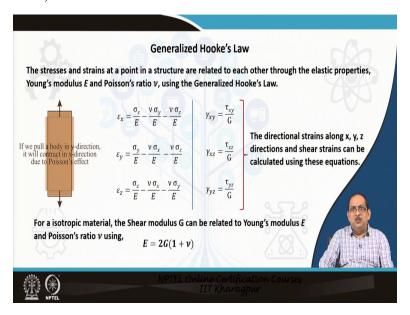
Now, let us consider a more generalized state of loading wherein it is indicated here in the figure that if we pull a body along the y-direction, it will tend to contract in the x-direction due to the poisons ratio effect. So, Poisson's ratio is the lateral contraction to the actual elongation. These stresses and strains at a point in a structure are related through the elastic properties Young's modulus and Poisson's ratio using the generalized law, generalized Hooke's law.
