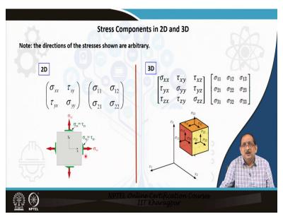
The stresses stress components in 2D and 3D systems are indicated in the slide and pictorially presented to understand each of the stress components in the tensor.
