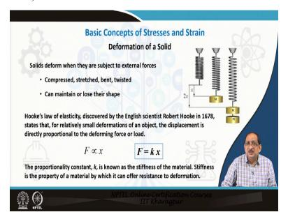
Now, let us first consider a simple spring-mass system. If the weight of mass M is hung from the end of spring, the spring undergoes an elongation of x, if the weight is doubled, the elongation increases to twice x. So, the solid bodies deform when they are subject to external forces; they are either compressed or stretched or bent or twisted. They can actually maintain their shape to some extent or lose their shape as well.
