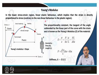
In the lower stress-strain region of the curve, linear elastic behaviour is exhibited, which implies that the strain is directly proportional to the stress contrary to the nonlinear behaviour in the plastic zone. The proportionality constant in this linear elastic zone is the tangent of the angle subtended by the linear part of the curve with the strain axis, and this proportionality constant is known as the Young's modulus of the material.
