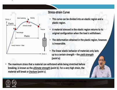
Now, let us discuss about the stress-strain curve. The stress-strain curve can be plotted from the data obtained from a tension test. So, here in we get we plot the stress-strain curve corresponding to a ductile material. So, there are a few important key points in this curve as well as two distinct regions.
