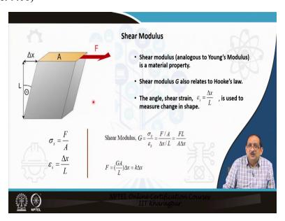
The shear modulus is another modulus analogous to the Young's modulus and it is an essential material property. The shear modulus also relates to Hooke's law; the angle known as the shear
