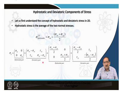
Now, the stress components can be classified as hydrostatic and deviatoric components of stress. Let us first understand the concept of hydrostatic and deviatoric stresses in a 2D system. The hydrostatic stress is basically the average of the two normal stresses as indicated here in the mathematical expression is the average of the two normal stresses. The state of stress actually can be expressed in such a way that we can obtain a hydrostatic part, and we can obtain a deviatoric part.
