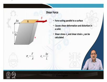
Let us define a shear force that acts parallel to a surface as shown in the figure, and it causes shear deformation and distortion in the solid object. So, this is the deformation and overall, there is a distortion in the shape of the solid object. Accordingly, shear stresses and shear strain can be calculated as indicated here in the slide.
