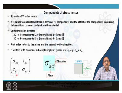
Now, let us, discuss the components of the stress tensor. Stress is a second-order tensor. A zeroth-order tensor is a scalar quantity, a first-order tensor is a vector quantity, and the second-order tensor is, for example, is stress. It is easier to understand stress in terms of its components and the effect of components in causing deformation to a unit body within a material.
