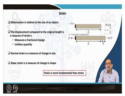
Next comes strain, when a cylindrical bar is subject to external tensile force, at one end, it may undergo a slight increase in length and decrease in diameter. The change in dimension is known as deformation. The average linear strain is the ratio of the change in length to the original length. So, strain is deformation relative to the size of an object.
