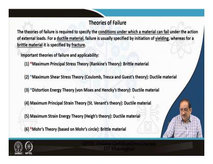
Failure theories are required to specify the conditions under which a material can fail under the action of a set of external loading conditions. For a ductile material, failure is usually defined by the initiation of yielding whereas, for a brittle material, it is specified by fracture. Some important theories of failure and their applicability is listed here.
