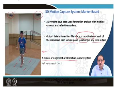
Let me reintroduce the marker-based 3-D motion capture system, which we had discussed in the earlier lecture. A typical arrangement of the 3-D motion capture system is shown in this figure. The 3-D motion capture system consists of multiple cameras and reflective markers, as can be seen in the figure. It comprises ten cameras mounted from the ceiling, only two are visible here and four force plates placed in the middle of the walkway.
