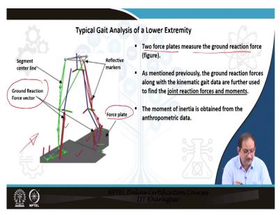
Now, a typical arrangement with the lower extremity model is shown in the figure. So, the two force plates measure the ground reaction forces. So, the force plate is indicated here, and it is giving us the ground reaction force vector.
