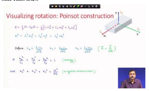
With a redefinition, we can recast the energy conservation constraint as an ellipsoid, and the angular momentum conservation constraint as a sphere, as presented in the above slide.
