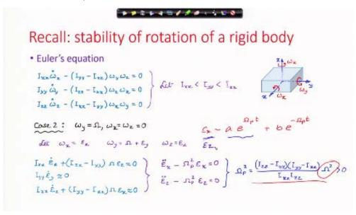
The linear stability of an unsymmetric spinning rigid body is revisited in the above slide.
