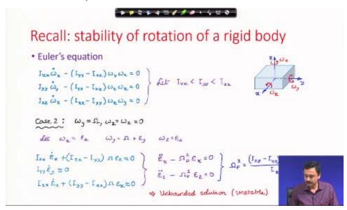
This linear stability analysis says that the spin about the intermediate axis has unbounded perturbation dynamics.
