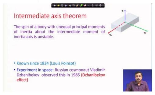
The intermediate axis theorem is stated in the above slide.
