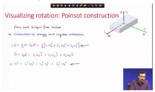
Poinsot devised an interesting way of visualizing the motion of a spinning rigid body. We start with the consideration that energy and angular momentum have to be conserved. These appear as constraints as presented in the slide above.
