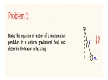
Let us start with most classical example the pendulum. We derive the equation of motion of the mathematical pendulum in a uniform gravitational field and determine the tension in the string. (Refer Slide Time: 12:24)
