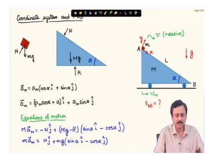
We choose a convenient coordinate system x-y which is fixed to the wedge. The second step is to draw the free body diagrams of the block and the wedge, which are shown above. The acceleration relations and the equations of motion are also shown.
