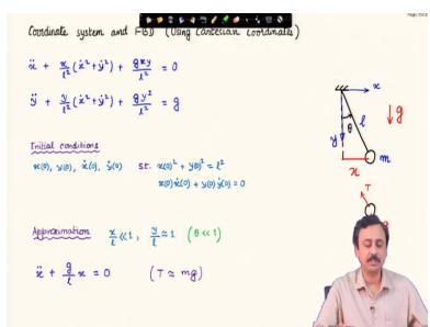
These equations are accompanied by constraints since x and y coordinates cannot vary independently. They must respect the constraint that the bob must always remain at a fixed distance I from the point of support. Thus, we have
