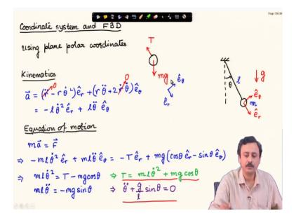
First step is to fix the coordinate system, and we choose to use the polar coordinates as shown above. The second step in the free body diagram, as shown. The acceleration vector represented in the polar coordinate system, as seen by an inertial observer, is
