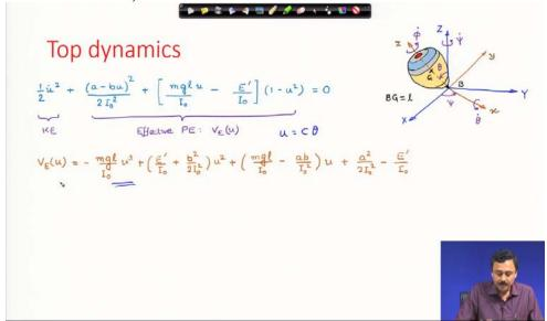
Using the integrals, one can reduce the dynamics of the top to a single dynamical equation, as shown in the slide above. Using the qualitative features of the effective potential energy expression, we study the dynamics of the top in the following 2 slides.
