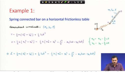
The first example is a spring connected bar on a horizontal frictionless table as shown in the slide above. The Lagrangian is also presented.
