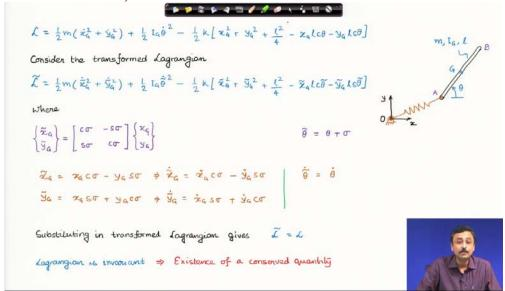
In the above slide, an infinitesimal symmetry of the Lagrangian is determined. This leads to the conclusion, based on Noether's theorem, that there exists a conserved quantity.
