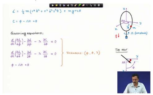
We introduce the constraint separately to enforce the condition that the bead actually moves on the hoop as shown above.
