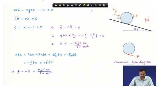
The above slide discusses the approach to determine the unknown friction force from the Lagrange multiplier.
