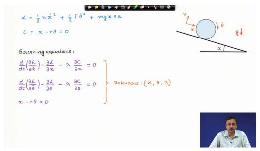
In order to do this, we break the rolling constraint and introduce it as a mathematical condition.
