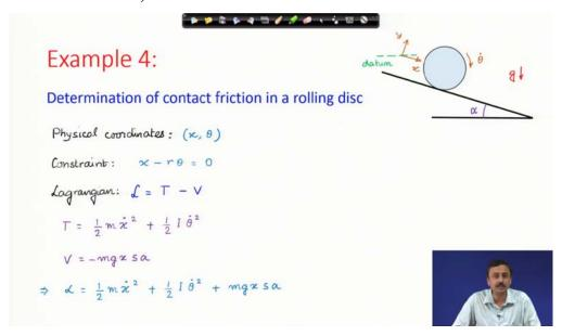
Now, we come to this rolling disc on an incline in a uniform gravitational field. We want to find out that friction force at the contact.
