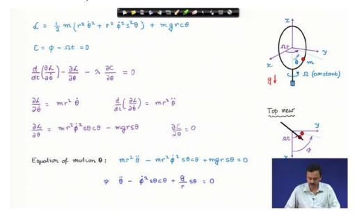
The equations of motion are then derives as shown in the 2 slides above. These equations involve the Lagrange multiplier.
