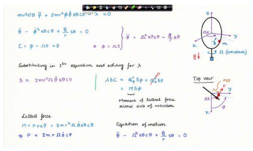
The above slide shows how the Lagrange multiplier is used to determine the lateral force and obtain the equation of motion.
