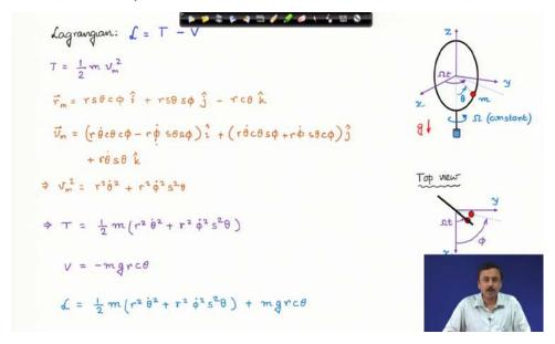
We introduce a new coordinate  $\phi$  as shown above. Thus, we break the constraint that the bead always remains on the hoop.
