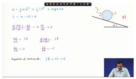
The equations of motion are derived in the above 2 slides. These equations involve the unknown Lagrange multiplier.
