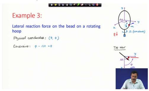
We will start with this example of bead on a hoop. The hoop is rotating at a constant angular velocity. I would like to find out the lateral reaction force on the bead from the hoop.
