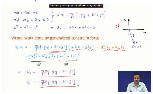
In the above slide, we determine the generalized constraint forces for the pendulum.
