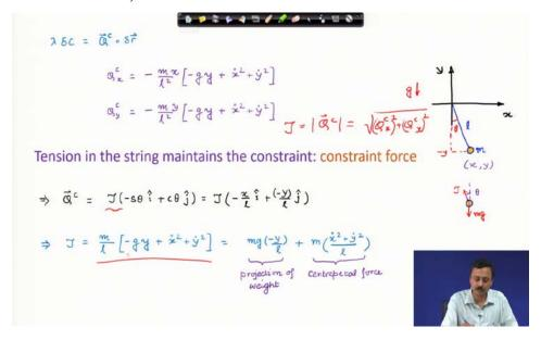
Using the generalized constraint forces, we determine the string tension.
