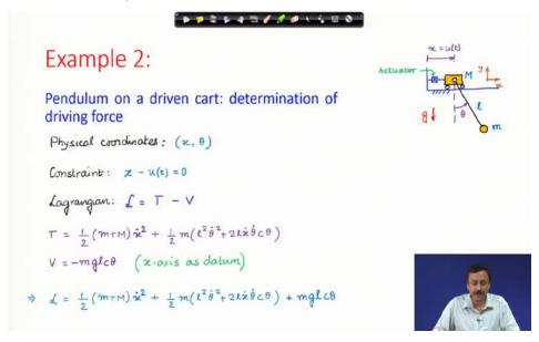
Let us then proceed to our second example, pendulum on a driven cart. We would like to find out the force required to drive the cart for a desired motion u(t) of the cart.
