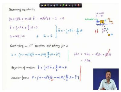
Finally, we obtain the actuator force as calculated above.
