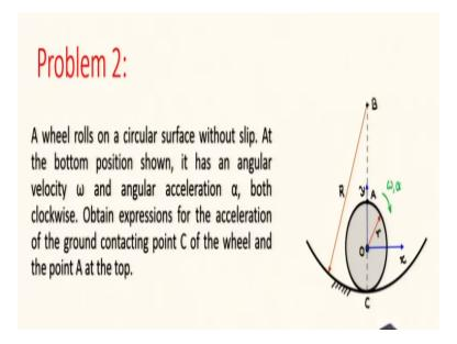
Let us extend this problem. Here the wheel is rolling on a circular track in a plane. It has angular velocity  $\omega$  and angular acceleration  $\alpha$  both clock wise. C is the point on the wheel which is currently in contact with the ground and A is the topmost point of the wheel at this instant.
