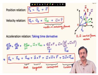
We first recapitulate the discussions in the previous lecture. The rotating frame xyz represented by the green frame in the figure has angular velocity  $\omega$  and angular acceleration  $\alpha$ . And XYZ is a fixed frame fixed with respect to distant stars. Now the position relation is
