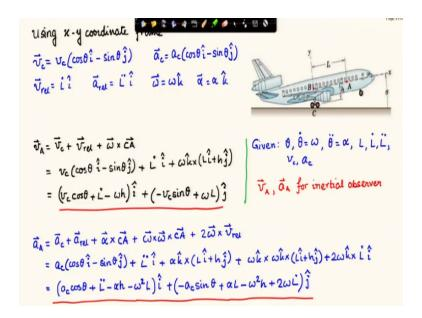
We will use the x-y frame that is given in the figure. I have written out all the given parameters that are specified in the problem we have to find out  $v_A$  and  $a_A$  as seen by inertial observer. We have represented all vectors in the x-y frame. Just plug in all the expressions and simplify to obtain
