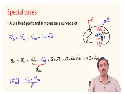
If B moves on a curved path of a certain radius of curvature as shown above the velocity relation is given by
