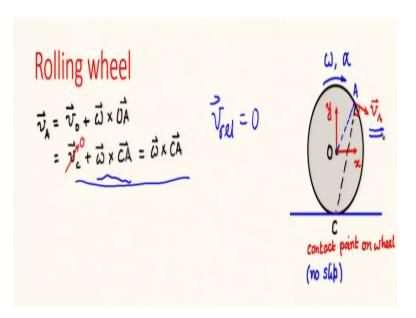
Now you can extend this to study acceleration or velocity of various other points on the wheel. For example velocity of A can be written in two ways as
