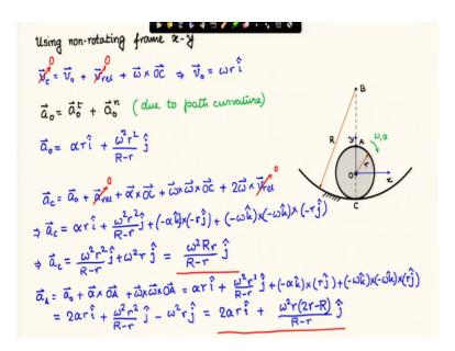
I take the non-rotating x-y frame and represent all vectors using it. From velocity relation
