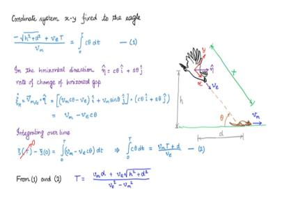
This is the first equation we have just now derived now let us look at this horizontal direction I have shown this unit vector in horizontal direction eta cap this is the unit vector in the horizontal
