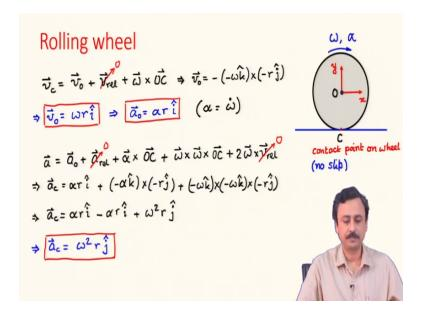
Consider the example of a wheel of radius r rolling on flat horizontal ground. The point C of the wheel is the point of contact, and I am assuming that this wheel is rolling without slipping. We consider a frame x-y I at the geometric center of the wheel and translating with it with the x-axis is always horizontal. Thus, this is a non-rotating frame.
