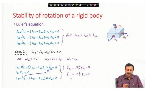
Let us move on to the second situation where we give the spin about the axis which has the intermediate moment of inertia.
