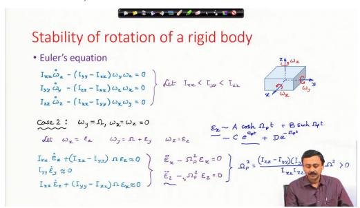
The disturbance dynamics equation in this case is presented above. From the nature of solution of these equations, we observe that one solution term represents exponential divergence. In other words, the disturbance in the x and z axes is going to exponentially diverge, implying that spin about the intermediate axis is unstable. This is sometimes known as the intermediate axis theorem.
