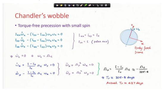
The equations of motion of torque-free rotational dynamics of an axisymmetric body is obtained from Euler's equations, as shown above. Using the known data of moment of inertia of the Earth, the precessional time period is estimated as 305.8 days. However, the actual value observed in 427 days.
