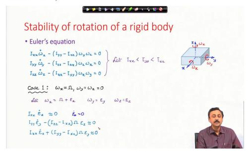
As shown above, the Euler's equations can be linearized considering the disturbance to be small, and dropping the second order small terms.
