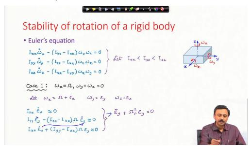
We time derivate the y-equation and use the z-equation to obtain the disturbance dynamics in the y-axis direction, as shown above.
