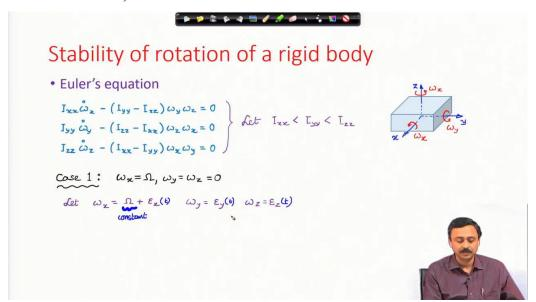
Consider a body as shown in the figure above. The Euler's equation for the rotational dynamics of the body can be written as shown. If the body is given a spin about the x-axis along with a small disturbance, the angular velocity vector components can we written as shown.
