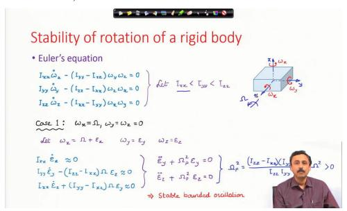
From the nature of solutions of the disturbance dynamics equations, we can conclude that if we give a spin about the smallest moment of inertia axis, the disturbances will remain bounded.
