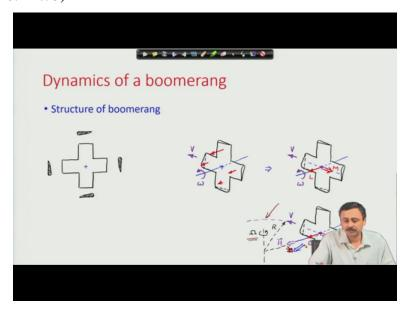
I have considered for simplicity this 4 arm boomerang as shown in the slide above. There is this crossed structure with 4 arms having aerofoil shape and note carefully how the aerofoils are oriented.
