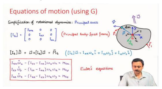
If we choose the x-y-z body-fixed frame as the principal frame of the body, the moment of inertia tensor becomes diagonal. In that case, we obtain the simplified equations of rotational dynamics which go by the name Euler's equations of motion.
