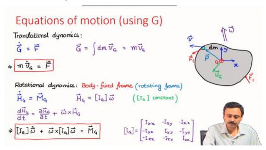
Finally, using a body-fixed frame, the equation of rotational dynamics can be written in terms of the center of mass G in the form shown in the slide above.
