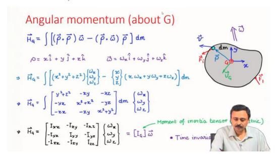
The calculation of the angular momentum vector leads us to the moment of inertia tensor calculated about the center of mass G, as shown in the slide above.
