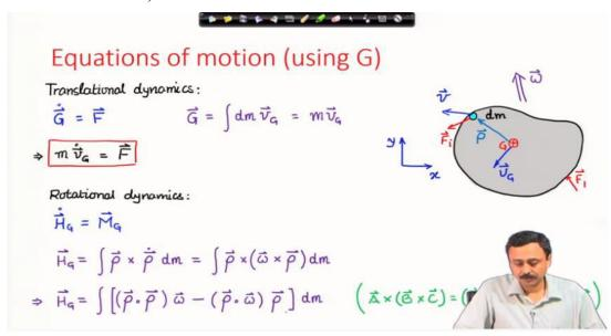
The above slide recapitulates the translational and rotational dynamics of a rigid body. The rotational dynamics is written for the center of mass of the body.
