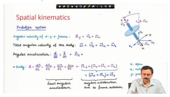
The above slide presents the calculation of the angular acceleration of the axisymmetric body.
