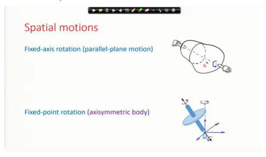
Spatial motions that we will consider will essentially be of 2 types, as shown in the slide above. When there exists a fixed rotation axis, it is called a fixed axis rotation or also known as parallel plane motion. The other is fixed point rotation of an axisymmetric body about a fixed point. Later, we will consider completely free motion of a rigid body.
