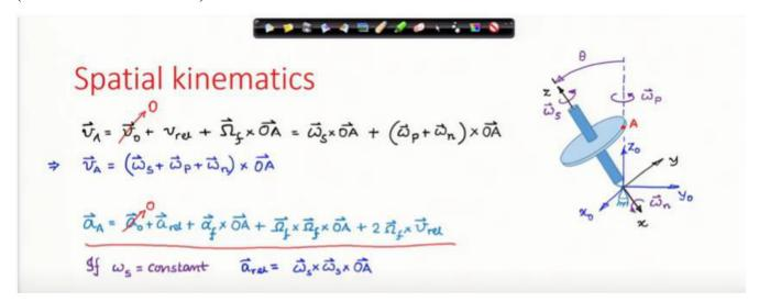
Consider now a point A as shown in red on the disk in the above figure. We can express the velocity and acceleration of A as presented above.
