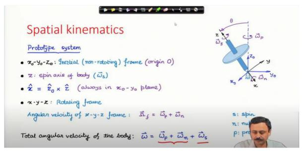
We are going to start with this prototype problem of rotation of a symmetric body about a fixed point. The parallel plane motion will be discussed a little later. In the above slide, I have shown in the figure an axisymmetric body rotating with a point fixed at the origin of the inertial  $x_0$ - $y_0$ - $z_0$  frame shown. The setting up of the x-y-z frame, and the angular velocity of the body is expressed in terms of the spin, precession and nutation angular velocities.
