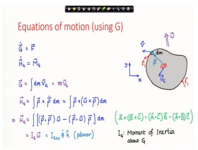
Let us look at the equation of motion of this rigid body about with the rotational dynamics equation or the angular momentum equation about G. So we have the translational dynamics equation which is the extended Newton's second law for the center of mass and the angular momentum equation about the center of mass. And you know that the linear momentum of the center of mass is defined this way the total mass times velocity of center of mass.
