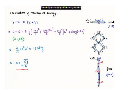
I have drawn the 3 states the starting state the intermediate state and the final state of the mechanism as it moves. This is in a uniform gravitational field there is no other active forces therefore the total mechanical energy of the system will be conserved. In state 1 which is the folded configuration initial and, state 2 is the final configuration which is the stressed configuration we have the total mechanical energy.
