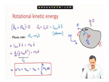
What changes the rotational kinetic energy? For that we have to look at the angular momentum equation in the planar case we are treating the thing for the planar case I take a dot product of the angular momentum equation with omega. For the planar case the moment about the center of mass moment of all forces about center of mass will be in the k cap direction therefore its representation will be M G k cap.
