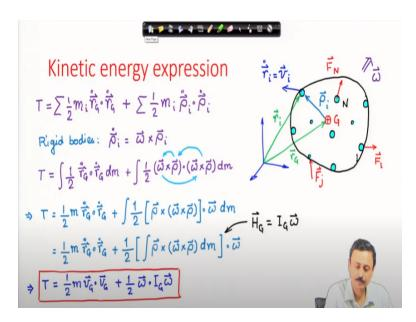
So this was the expression of kinetic energy of translation of center of mass and kinetic energy of motion about the center of mass kinetic energy because of motion of the particles about the center of mass. Remember that rho i dot is the relative velocity of the ith particle with respect to the center of mass. Therefore the second term in the kinetic energy expression gives us the kinetic energy because of motion of the particles about the center of mass.
