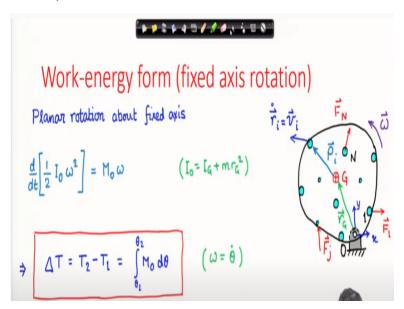
So this is our expression now here. I can write omega as theta dot k cap this which I had written previously. The omega vector was theta dot k cap because this is linear motion and in that I can write it like this. Therefore this d t omega vector d t this is what I will have here and that turns out to be theta dot d t k cap. And everything is in k cap direction actually. Everything here is a scalar finally it has reduced to a scalar.
