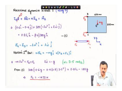
Next we move to determine the forces in that member that connects at C the member D C for that I am going to write the rotational dynamics of this plate in the second configuration or state 2 and I will use the point B. Why I use the point B? Because the angular momentum equation about B is the moment of inertia of the plate about B times angular acceleration + B G cross mass of the plate times acceleration of B that is equal to the net moment about B.
