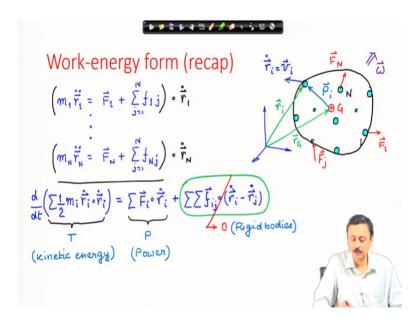
Just to recapitulate what we have discussed for a system of particles because this is what we are going to extend to rigid bodies. Here we had written out the Newton's second law for all the particles we had n particles suppose we have n particles. We write down the Newton's second law for all these particles. And we had taken dot product of each of these equations with the corresponding velocity of that particle.
