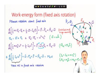
If you consider planar rotation about a fixed axis then there are some simplifications possible that I was mentioning. Now velocity of center of mass can be written as omega cross r G and you note what is r G here? This is r G vector from O to the center of mass velocity of center of mass is omega cross r G and therefore velocity of the center of mass square is omega square r G square and omega has this form.
