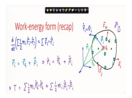
And then we had looked at the decomposition of the kinetic energy expression. And we have found that the total kinetic energy of this system is equal to the kinetic energy of translation of center of mass with all the mass concentrated at the center of mass as if center of mass is a point particle. And we are writing the kinetic energy of the point particle this is one term in that expression of total kinetic energy.
