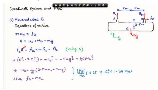
The coordinate system and the free body diagram are shown in the slide above. To begin with, we consider that wheel B is powered. Then the calculation to determine the maximum acceleration is presented.
