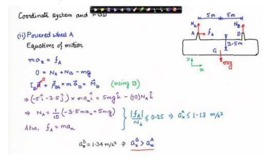
The calculation of maximum acceleration when wheel A is powered is shown above. It is found that we can achieve higher acceleration when wheel B is powered.
