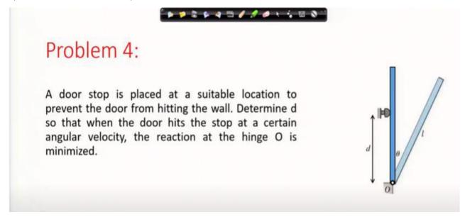
A problem related to the positioning of a door stop is shown in the slide above.
