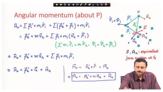
The calculation of angular momentum about an arbitrary point P as shown in the slide above.
