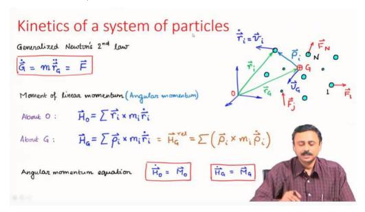
The above slide recapitulates the generalized Newton's second law for a system of particles. The definition of moment of linear momentum or what is also known as the angular momentum is also presented above.
