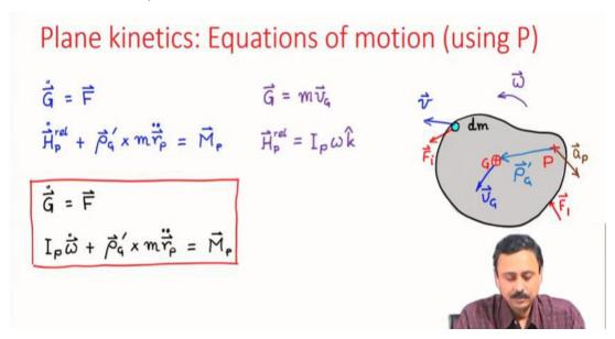
In the first case when P belonging to the rigid body is not fixed in inertial space, the equations of motion of the body are as shown above.
