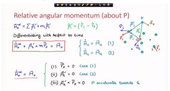
We obtain 3 special cases as shown above for which the angular momentum equation takes a particularly simple form. These cases are: (i) when P is a fixed point in inertial space, (ii) when P is the center of mass of the system, and (iii) when P is accelerating towards/away from the center of mass.
