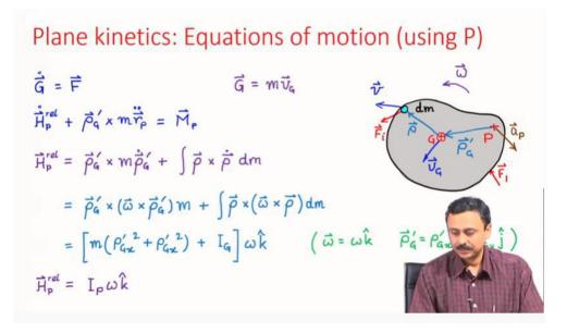
The above slide shows the calculation of the relative angular momentum of the body about the point P fixed to the body.
