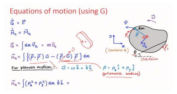
When we go to rigid bodies the summation of linear momenta just gets converted to an integral as shown above. We can similarly express the angular momentum about the center of mass as an integral as
