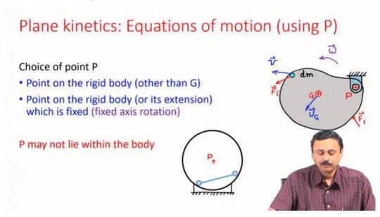
Now we consider a general point P. There can be 2 possible choices of P. The point P can be a point on the rigid body which is not G, or it can be a point on the rigid body or its extension which is fixed.
