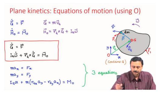
Now we look at the equations of motion of plane kinetics of a prismatic rigid body about a fixed point O. This is presented in the slide above.
