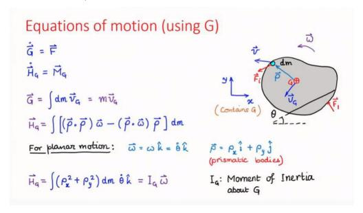
The angular momentum about the center of mass of a lamina is presented in the slide above.
