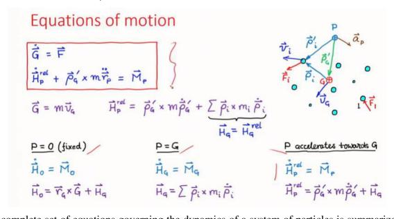
The complete set of equations governing the dynamics of a system of particles is summarized in the slide above.
