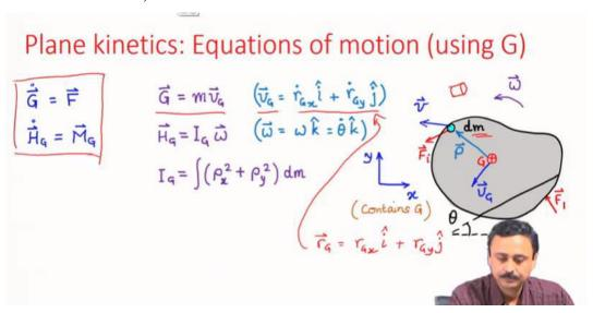
The complete equations of motion of a lamina in planar motion is presented above.
