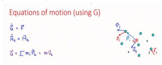
Now let us go back to equation of motion that we have derived about G now for a system of particles.
