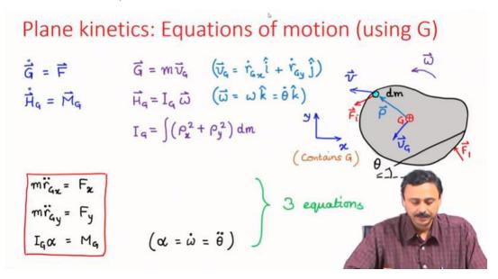
The 3 scalar equations obtained from the vector equations are presented in the slide above.
