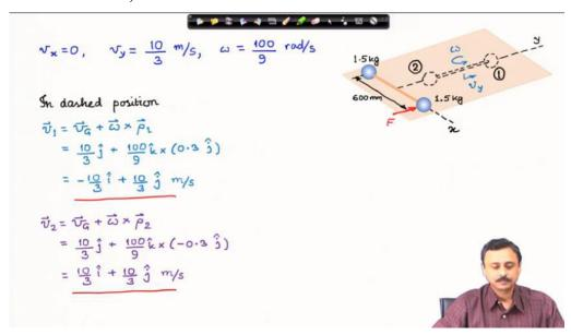
Finally, using these two information, we calculate the velocities of the two balls as presented in the slide above.
