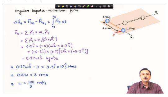
Now we look at the angular impulse momentum relation as shown in the slide above: the change of angular momentum about the center of mass is equal to the moment the impulse of the moment about the center of mass. Using this, we get the angular velocity of this system. Now the angular velocity of the system tells us how the system will change its orientation as time
