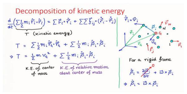
As shown in the above slide, the total kinetic energy of the system of particles is sum of of 2 parts: (i) the kinetic energy due to the motion of the center of mass with all the mass concentrated at the center of mass, and (ii) the kinetic energy of all particles moving relative to the center of mass.
