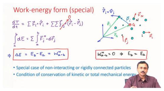
In the case when potential forces are present, we can define potential functions corresponding to each force, and the work done by such forces can be expressed as the negative of the change in the potential energy of the system as
