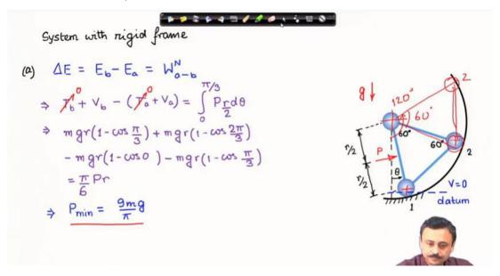
The solution is presented in the slide above using the work-energy relation to determine  $P_{min}$  required to take the system to the configuration with  $\theta$ =60 degree.
