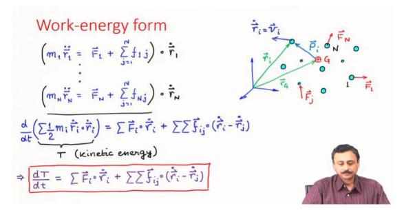
Next we will look at the work energy relation for a system of particles. First, writing out the Newton's  $2^{nd}$  law for the individual particles, we take dot product of the  $i^{th}$  particle equation with the velocity vector  $dr_i/dt$ , and sum over all particles as shown in the slide above. This leads to the rate of change of kinetic energy of the system as
