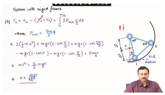
In a second part of this problem we have to find out the common velocity of the 2 particles 1 and 2 when  $2P_{min}$  is applied in place of  $P_{min}$ . The solution is again approached using the work-energy relation as shown in the slide above.
