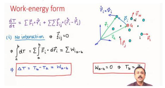
We consider two cases. The case (i) of no interaction between particles (i.e.,  $f_{ij}$ =0) is shown in the slide above. This leads to the work-energy relation
