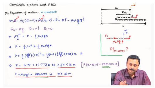
The coordinate system and free body diagram for the moving part are shown. The moving part of the chain constitute the system to which. This is a variable mass system.
