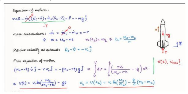
The coordinate system and free body diagram are shown in the slide above. From the mass conservation equation, we can find the fuel burn-out time as shown. By integrating the master equation, we determine the velocity at any time t, and the velocity at burn-out is also determined.
