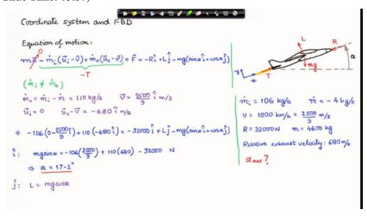
The coordinate system and free body diagram are shown in the slide above. The acceleration term in the master equation for this problem drops out since the aircraft is flying at a constant velocity. We plug in the values of the various terms in the master equation and obtain the maximum elevation angle of the aircraft as shown above.
