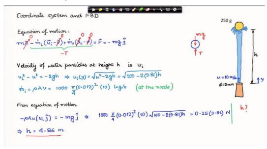
We consider our system as the ball and its surroundings. Since the ball is stationary at the balanced position, its velocity is zero. We consider that the water particles enter the system boundary at a certain velocity and come to momentary rest against the ball. This leads to some simplification of the master equation for this case, as presented in the slide above. The detailed solution is also presented in the above slide.
