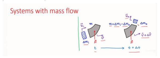
Now to derive the equation of motion of system with variable mass, we consider a body which ingests and ejects small quantities of mass as shown above in a short duration of time. The absolute velocities of the body and the two mass blobs are shown. The body is acted upon by a non-impulsive force external force F.
