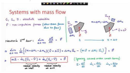
We write down Newton's second law for this system, as shown in the slide above and take the limit of the time interval to zero. Dropping second order small quantities, we obtain
