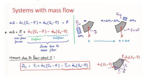
We rearrange the master equation to bring the additional terms on the left hand side to the right hand side, as shown in the slide above. These additional terms represent the flow forces due to inflow and outflow. One can also calculate the moment of the flow forces on the body about a fixed point as shown in the slide above.
