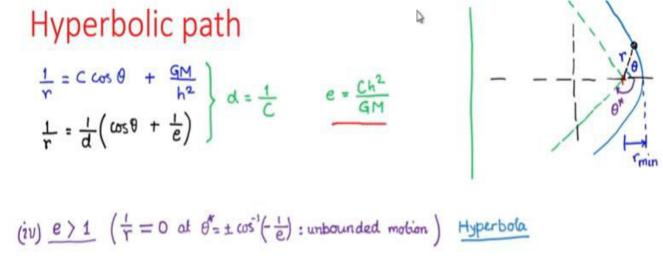
The characteristics of a hyperbolic trajectory is shown above.
