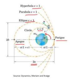
The above slide puts together all kinds of possibilities of motion of a particle under a central force field.
