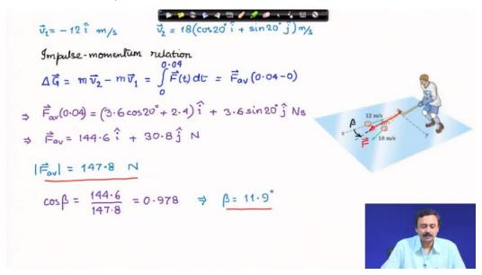
The detailed solution is presented in the slide above. This involves application of the vector form of the impulse-momentum relation as demonstrated above.
