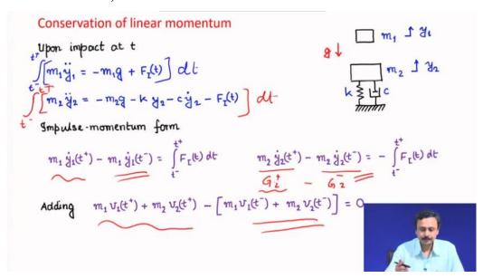
Let us try to understand this thing with this example of a mass falling on top of a mass spring dash spot system in a uniform gravitational field, as shown above. The equations are written, and integrated individually to obtain
