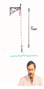
This example is about a bungee jumper who uses a cord whose free length is 15 meter and reaches a maximum jump depth of 22 meter. This depth is measured from the point of jump as I have shown  $X_{max}$ =22 meter from the point of jump. There are 2 acceleration regimes
