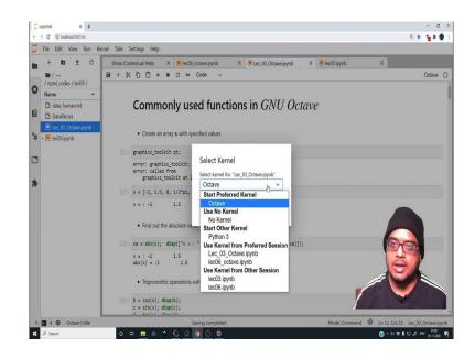
In this particular case, we have used the environment of Jupyter Lab and used the Kernel Octave, Jupyter Lab allows you to use multiple Kernels. You can program in Python, you can program in Octave, you can program in Julia. You can in fact program in MATLAB also using Jupyter Lab. Jupyter Lab provides you a nice way of writing down documentation as you progress in the program; things like bullet points, things like equations ok.
