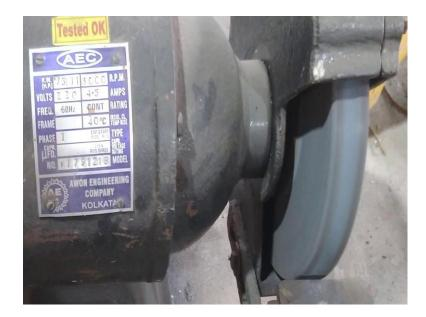
And the fact of the matter is I checked the label of the bench grinder and it did say that the bench grinder runs at 3000 RPM and not 15000 RPM, what could be the reason it runs at 3000 RPM? The reason is over here instead of having 4 poles it has 2 poles.
