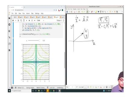
So,  $\dot{x} = Ax$ , ok. So, if we know that the space, the two-dimensional space has eigenvectors  $v_1$ ,  $v_2$ ; then it means that, any vector in this space can be written in terms of a linear combination of these two vectors. So, *x* can be written as  $c_1v_1 + c_2v_2$ . And this vector is not a velocity vector or something like that; it is the pair of terms (*x*, *y*) and in that quantifies the vector in the x-y plane, do not be confused with the velocity vector over here, ok.
