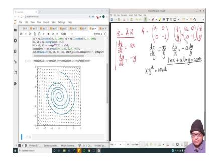
So, now, let us move ahead to find out the behavior of a prototypical linear system. So,  $\dot{x} = Ax$ , where A is given as a, (0, 0, -1), ok. So, let us look at how in this particular system would look like over a matrix, which looks something like this. So, when we have this, we can write  $\frac{dx}{dt} = ax$  and  $\frac{dy}{dt} = -y$ ; this is because  $\dot{x}$ ,  $\dot{y}$  will be equal to (a, 0, 0), (-1, x, y).
