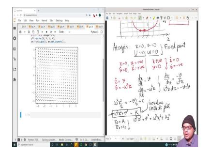
And actually, we can write this as  $\omega^2 x^2 + v^2 = K$ . Now, what is the value of the constant? It depends on the initial condition. If we choose  $x_0 = k_1 \& v_0 = k_2$ ; then we have  $\omega^2 x^2 + v^2 = \omega^2 k_1^2 + \omega^2 k_2^2$ .
