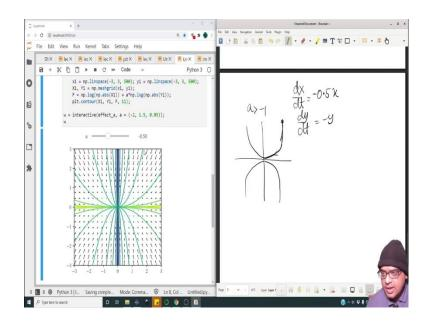
So, when a is greater than 0.1, say a is 0.5; then  $\frac{dx}{dt} = 0.5x$ , well  $\frac{dy}{dt} = -y$ . So, x is attracting slower than y. So, the trajectories are faster in the y-direction and then slower at the x-direction. So, the trajectories travel towards the x-axis faster than in the y-axis.
