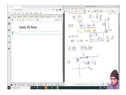
So,  $\dot{v}$  becomes  $\omega^2 x$ . So, this we have two equations. So,  $\dot{x} = v$  and  $\dot{v}$  becomes  $\dot{v} = -\omega^2 x$ . In the case of 1 dimensional equations, we had an idea of a vector flow.
