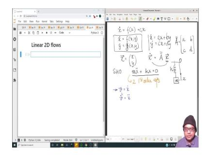
Now, when f(x, y) and g(x, y) are linear functions of x and y; meaning  $\dot{x}$  is some  $c_1x + c_2y$  or more generally we can say  $\dot{x}$  is ax + by and  $\dot{y}$  is cx + dy. Then such kinds of flows are called as linear flows. And the reason why we study linear flows is that, the behavior of linear flows will give us more insight into the behavior of non-linear flows; it holds the key towards understanding what the behavior near various fix points will be.
