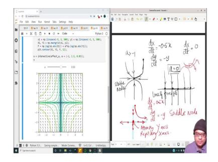
Now, when a group becomes larger than 0, see what happens;  $\frac{dx}{dt}$  is some say 0.5x and  $\frac{dy}{dt} = -y$ . So, x is growing exponential in time. So, if I have a point on the x-axis, it is growing exponential in time. So, it is going away from the origin; but a point on the y-axis is nevertheless attracted towards the origin, ok. So, this particular fixed point it is attracting in the y axis, but repelling in the x-axis.
