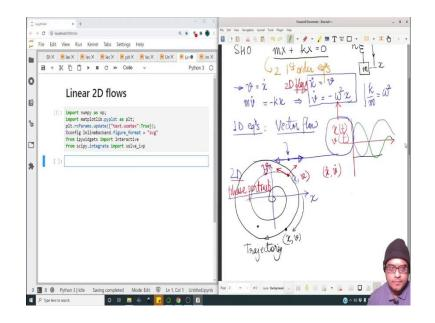
So,  $\dot{x}$  and  $\dot{v}$  are like telling us how this point in this plane would move given this kind of flow. So, this is called as a 2D flow and depending on this right-hand side, it would tell us how this point would move. If at a certain *x* and *y*,  $\dot{x}$  is positive and  $\dot{v}$  is also positive and obviously it will, this point will tend to go towards a higher *x* and a higher *v*.
