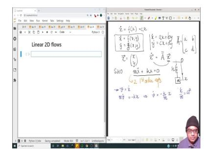
So, if  $v = \dot{x}$ , we can write  $m\dot{v} = -kx$  or essentially  $\dot{v} = -\frac{k}{m}x$ . Where  $\frac{k}{m}$  we can sub, we can I mean if you remember your high school physics,  $\frac{k}{m}$  is like the  $\omega^2$  parameter of an oscillator, ok. We are not going to discuss about how this comes into being, but it is related to the frequency of oscillations.
