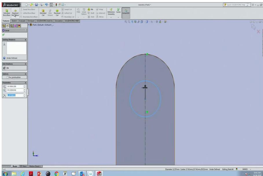
Maybe a circular hole we would like to have and it supposed to pass through centre line. So, now, zoom in this portion, use smart dimension; pick the first one control button, centre line, click ok, then make it 0.
