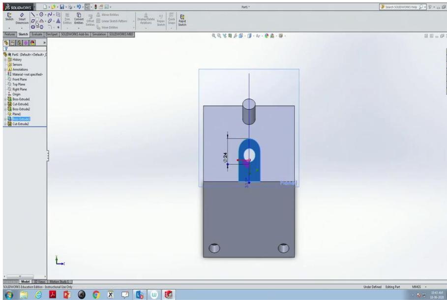
Now, we would like to have something like a slot on this portion, on this surface only. So, something like a rectangular slot, a small portion I would like to have. For that purpose, what I am going to do? Construct a rectangle, done.
