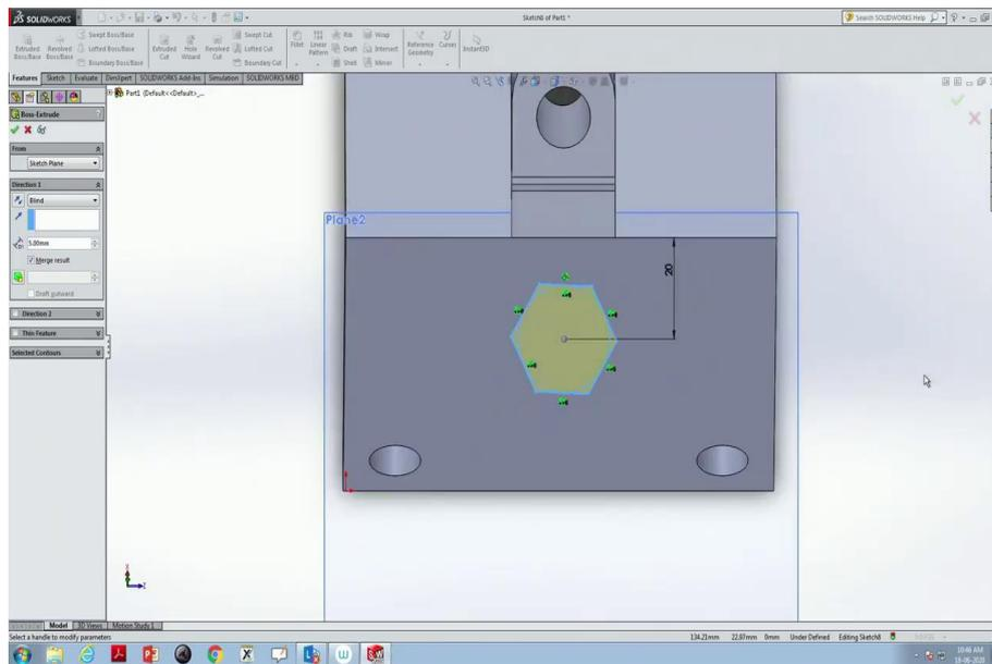
Now, I would like to use smart dimension, this point and this point supposed to be at 20 units of distance, done. Now, remove that circle, ok. Now, remove that circle oh its dimensions are there; click this, go to features, extrude boss base.
