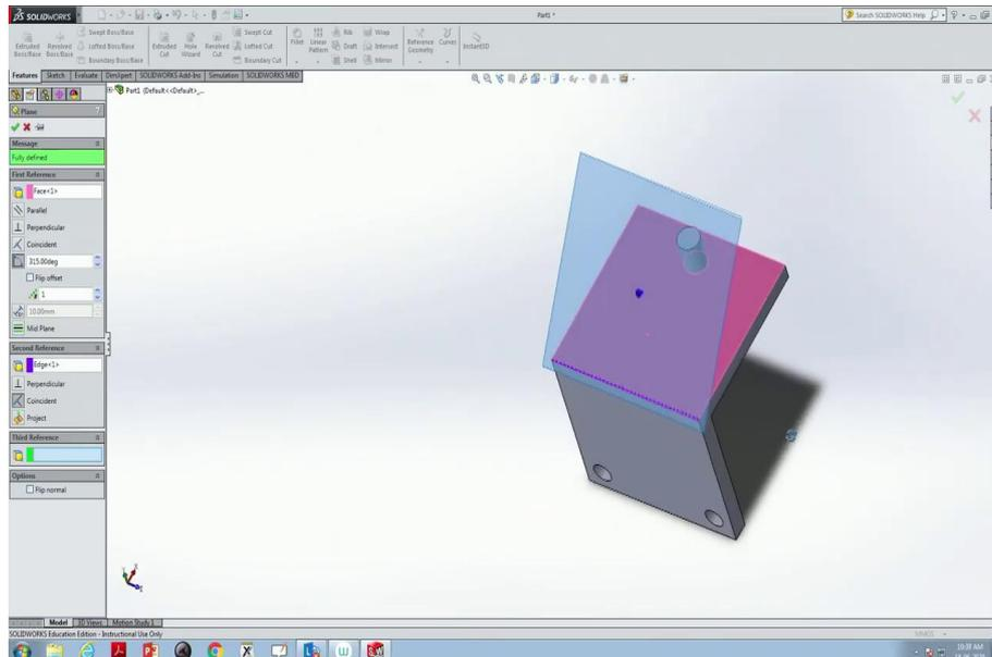
Now, on this surface, we would like to have an inclined surface on which there will be the additional thing. So, to construct the difference plane, first, we will go there click; this is the object and with respect to that same inclination angle we would like to have. So, for that purpose, pick the second reference and change this angle to something 315 degrees.
