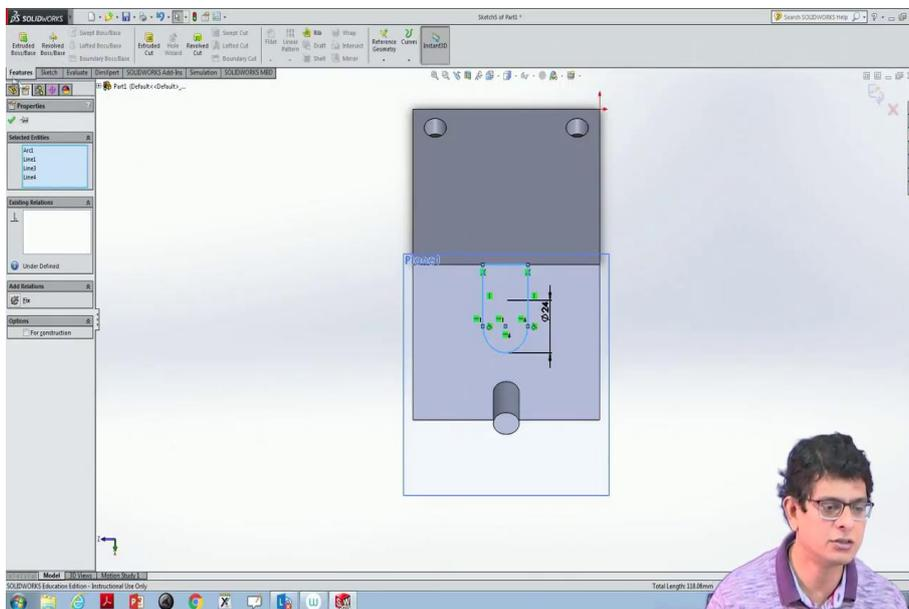
For example, I would like to construct a circle here and that supposed to have a unit of 24 diameters. And from there I would like to construct one more line passing through that and tangent to this line. Now, I will go ahead trim this object, click ok; then pick this one, this line, this one to extrude the object, extrude boss base.
