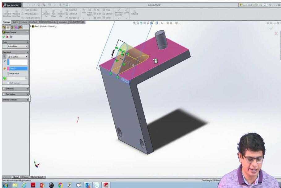
Now, if you are seeing, normal to that surface I can construct a plane. Now, we would like to have this entire constructed object touching the other side of that surface. So, I would like to have a extrude of this object entirely touching this surface; to do that what I have to do? Reverse the direction, so there is up to the surface; so click up to the surface, control button then clicks this surface.
