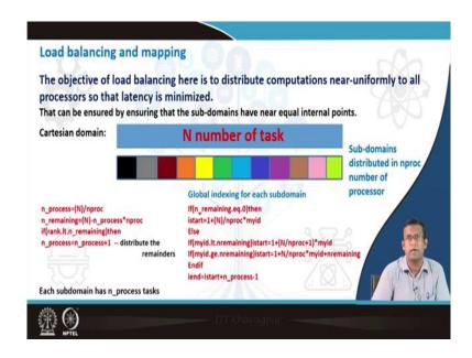
The next important part will be load balancing. What I told you earlier is that the main domain is such a way that nearly equal numbers of cells go to each sub domain and nearly equal numbers of tasks are going into each of the CPUs. We have to find an algorithm by which we can give nearly equal amounts of work to each of the CPUs. So, the idea of load balancing is that near uniformly the tasks are balanced to all the processors, so that the latency is minimized.
