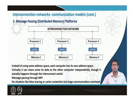
So, we look into Distributed memory platforms or message passing based platforms. There is an interconnect network and many processors with their own caches and own memories are connected to the same interconnection networks.
