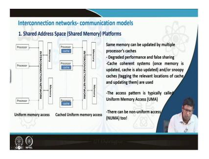
So, you should also look into shared memory or shared address space machines, that there is one interconnect network which is connected with many CPUs and this can be through an interconnect meter, this can be through a shared address connected also and memories are connected with the interconnect network.
