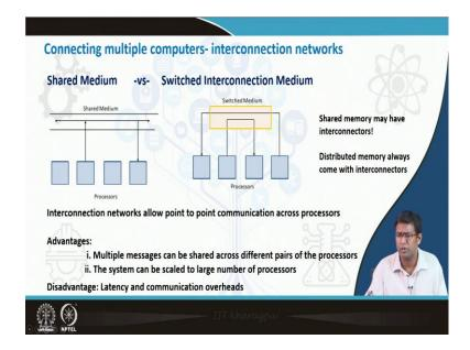
Now, we come to multiple computer system. So, how multiple processors can be connected and there are two typical arrangements one is called a shared medium that there is a single bus in which many processors are connected.
