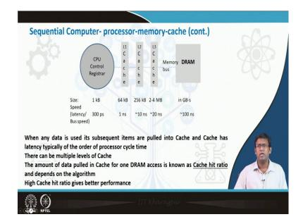
So, if we look into a sequential computer architecture, it's not a processor memory arrangement rather it's a processor cache memory arrangement. So, there is a CPU controller register, this register has a very small memory .Any variable coming from caches or dram is directly loaded to register and CPU can only work on the registered variables. The size of the memory is 1 kilobyte which is very small and latency is very small also it is 300 picoseconds.
