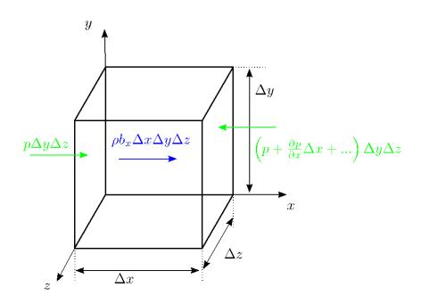
Fig 1: A fluid element for derivation of Euler equation of motion
