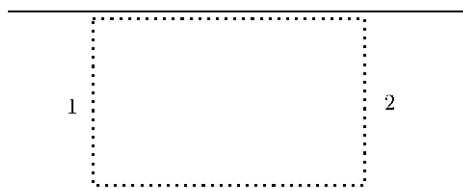
Figure 2: Section of a conduit with fluid flowing from left to right, with the control volume in consideration outlined using dotted line
