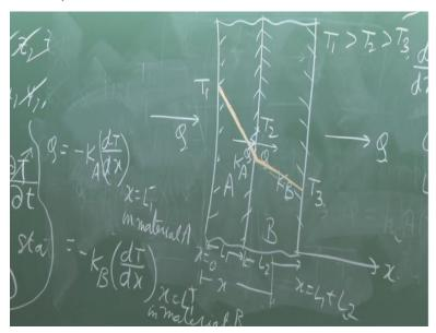
So, this will be steep this will be flat and if we apply our physical sense then also it is true that here since the thermal conductivity is low so this side at the end of this plate the temperature is less then this that means it cannot sense a temperature very close to this but since the thermal conductivity of this plate or this wall is high that means this side down stream side this outlet side or this face the temperature is close to this inlet face.
