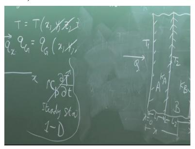
That heat which that means the qualitative picture of the slope that heat which is coming here from this side of this material A to this surface and the same thing flowing here is same Q so therefore one can write Q is equal to - k, dt by dx, KA at A. That means mathematically I write x, L1 - that means in material A that means L1 - means from this side must be equal to - KB into dt by dx at x is equal to L1 + means in material B.
