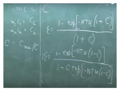
That means the capacity rate or simply the capacity and m dot c m dot c C c is the C c and m dot h c h is equal to C h and if I define C as the ratio of C min/c which may be either this by this that means this by this or this by this depending upon the case. In that case the expression will be very simple it looks like simple expression remain same 1- exponential minus NTU where NTU is minus uA. Sorry, not minus, sorry.
