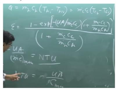
In terms of this quantity. Clear? Now here m dot c C c is the minimum heat capacity. Now this term minus u A/m dot c minimum is known as number of transfer unit NTU which is a dimensionless term overall heat transfer coefficient, surface area of the heat exchanger divided by m dot into c minimum. Now if you can ask me the question you should ask this question to me. Without gossiping or chatting with your friend at the back sir, if the hot fluid is the minimum fluid what could you have done?
