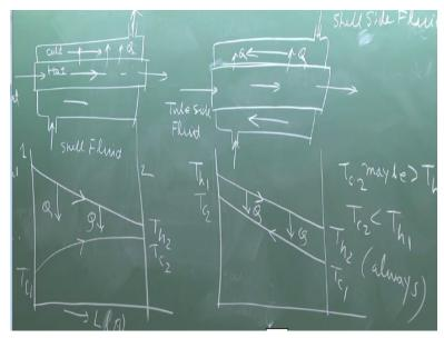
Now, I will go to the heat exchanger. Now this is Tube Fluid. And this is Shell Fluid. Now this is a Parallel flow arrangement and this is a Counter flow arrangement. This is the Tube Side fluid flow. And this is the Shell Side Fluid. Now this is a parallel flow, as I told that flows in the same direction; this is a counter flow. Now we will go for analysis for which we take a very simple configuration of one tube.
