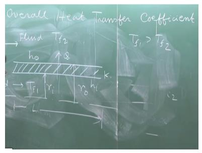
Let us consider this case again what we read earlier that there is a pipe I am drawing the symmetric part from the axis which has a fluid flowing through this pipe simply going back to the first few lectures, introductory lecture of heat transfer which I taught you. Fluid at a temperature of Tf1 and there is another fluid flowing through outside fluid which is at Tf2 that means the ambient fluid.
