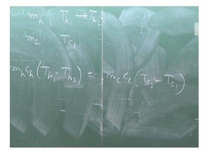
Now let us consider a situation like this, you have a duty fixed that means you have cool a hot fluid from Th1 to Th2 known. And you know that your cold fluid flow rate requirement available is this. And the cold fluid temperature available is this Tc1 which is usually the ambient temperature. So immediately a boy of class 8th will write mhch (Th1 – Th2) is equal to mcCc (Tc2 – Tc1) because entire heat exchange is insulated so from energy balance you will write and find out Tc2.
