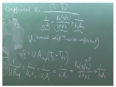
Then if you remember correctly than Q is equal to Tf1 - Tf2 that is overall temperature difference potential difference divided by 1 upon hiAi, if Ai is the inner surface area that means twice pie rl into L. I am not writing in this fashion, inner surface area plus if you remember ln(ro/ri) divided twice Pie kL plus 1 by hoAo which is twice pie ro into L that is outer surface area.
