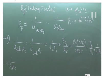
And that is expressed by a fouling factor denoted by R comes from the resistance this fouling factor expressed in terms of a resistance R and which his defined as—and because of that what happens thermal resistance enhances therefore the overall heat transfer coefficient gets reduced. Because thermal resistance is 1/u tens a reference area and therefore it is the heat transfer terminology in the practice that define the u dirty.
