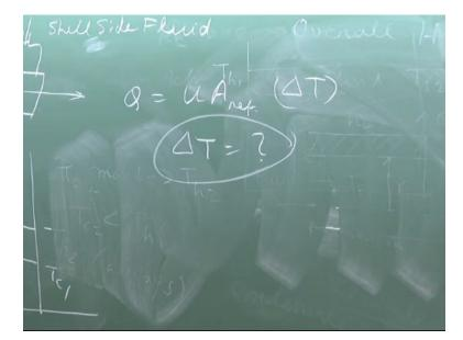
So, if I write this here for heat exchanger Q is equal to u - let us take overall outer surface area uA or inner surface area, reference area A0 or Ai does not matter Delta T, what Delta T? This is a big question this Delta T changing. For example, in a parallel flow it is Th1 – Tc2 and not Th2 – Tc2, so Delta T is maximum at the inlet. In case of parallel flow this goes on decreasing which Delta T. Which I will take?
