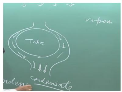
Just I tell you certain things that in the circular tube, usually what we use, it looks like that. If tube is horizontal like this a horizontal tube and if the vapour flows like this either push vapour or vapour flow, flow with a gentle velocity, then what happens it looks like this, the film grows; the picture is like this and tickles down the surface of the; this is the tube, tickles down the surface; this is the film, tickles down the surface of the tube.
