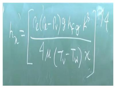
Then you get hx equals to K by delta. That means here I write hx is equal to this thing will go top, K by delta. That means K4 that means this will come, you just see rho l, rho l minus rho v into g hfg into KQ divided by this one will come 4 mu Tv minus Tw into x whole to the power 1/4. What happens K by delta, that means hx will be K by delta. This will be K inverse this and K4, I make and take it under one-fourth root, so it will be KQ, clear, Okay. **(Refer Slide Time: 44:50)**
