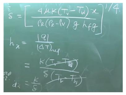
Therefore, I can write that delta is equal to 4 mu K Tv minus Tw x divided by rho l, rho l minus rho v g hfg, g is the acceleration due to gravity, hfg is the enthalpy of condensation whole to the power 1/4. This was Nusselt derivation for the growth of film, which is proportional to the fourth power of the x. If you compare it with the growth of boundary air over a flat plate in laminar flow.
