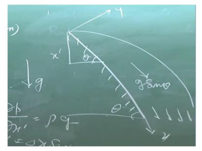
If the plate is inclined with an angle theta with the horizon, it is simply school level thing. So therefore, this is y and this is x, but g is in this direction. So entire thing will be changed by an effective g, g sine theta.
